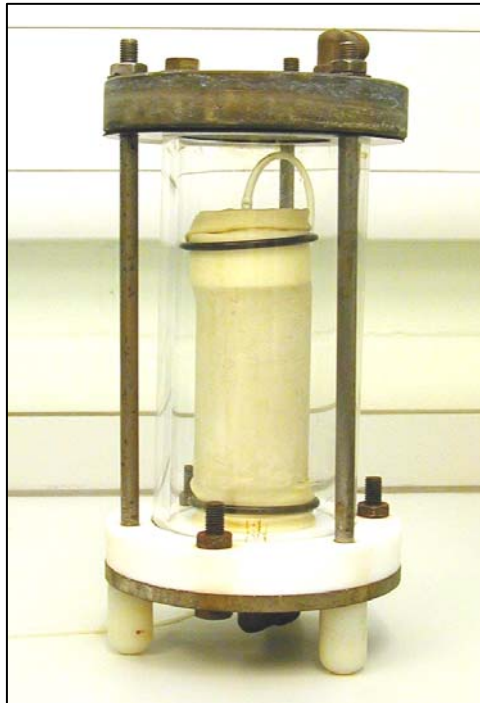
Figure A3.12 Triaxial cell apparatus containing a sample wrapped in PTFE and latex
