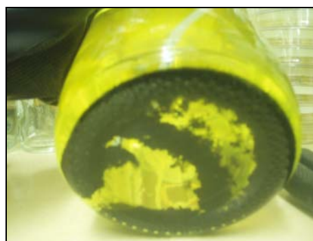
(a) (b) (a) London Clay air dried and ground prior to use in the biodegradation tests; (b) dark coating after 10 months incubation
