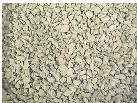
(a) (b) (a) London Clay air dried and ground prior to use in the biodegradation tests; (b) dark coating after 10 months incubation
