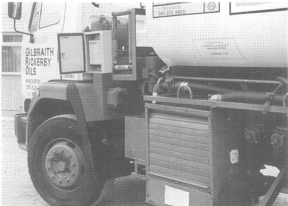
Figure 1 Side view of tanker showing meter box and litre counter/control box
