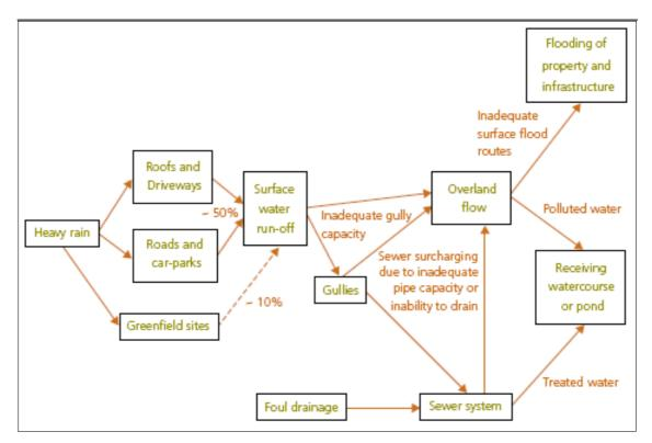
Figure 5.2 Main routes for discharge to receiving waters. Source: Great Britain (2008)
