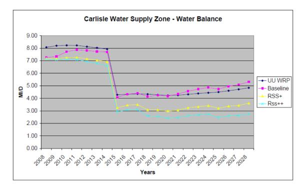
Figure 4.3 Water balance in the Carlisle Water Supply Zone
