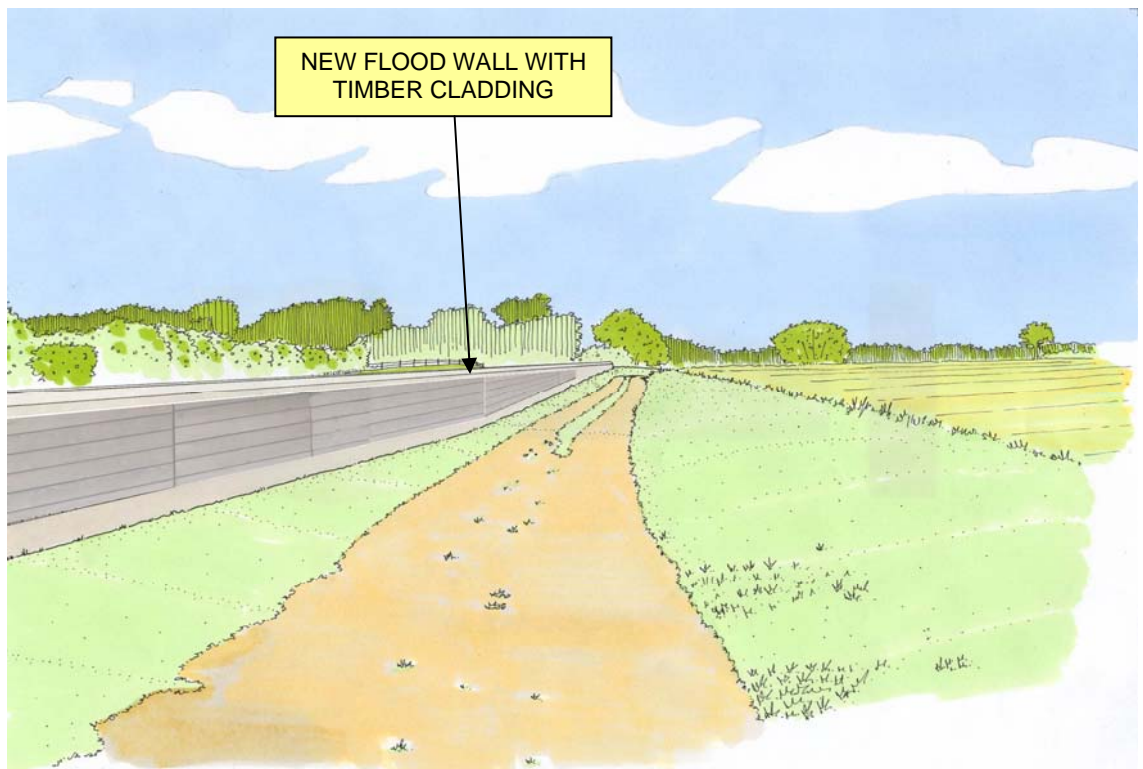
Plate A7.16 Visualisation of New Flood Wall through Reach 11 adjacent to the Nottingham/Derby Railway Line.
