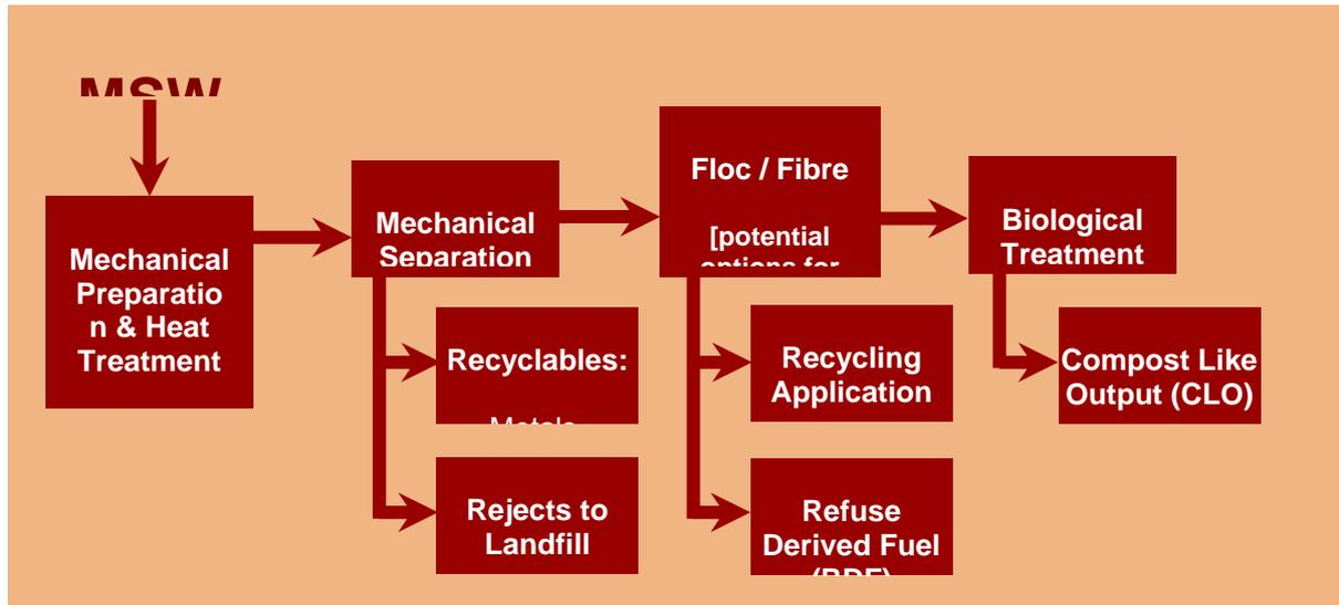
**Figure 1: Mechanical Heat Treatment Schematic**
