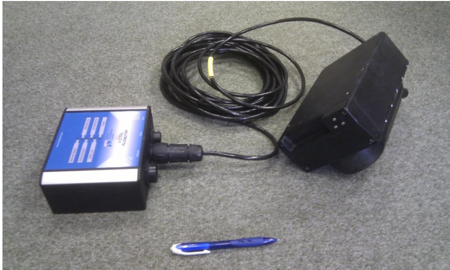
Figure 5: Tritech Gemini hardware including the transducer (right) and topside communications and power unit (left).
