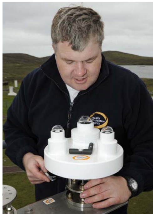
Figure 1: Solar radiation monitoring system head unit
