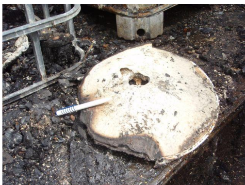
Figure 5 – remains of cardboard filter
