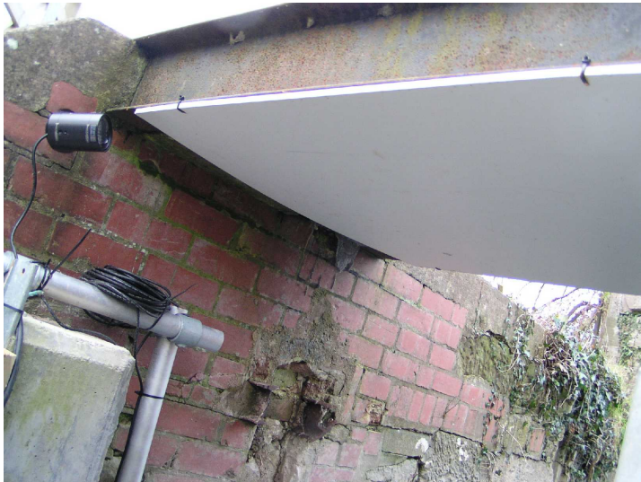
Figure 18: Infrared light was reflected off a white polypropylene sheet positioned above the fish pass exit
