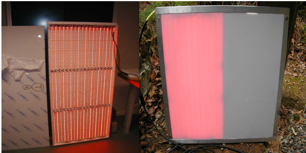
Figure 3.3: LED light panels under construction and complete
