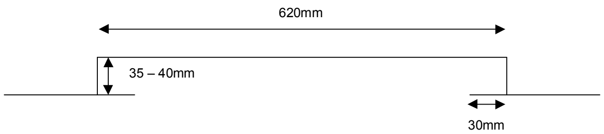
Figure A1.1: Side runner detail and dimensions
