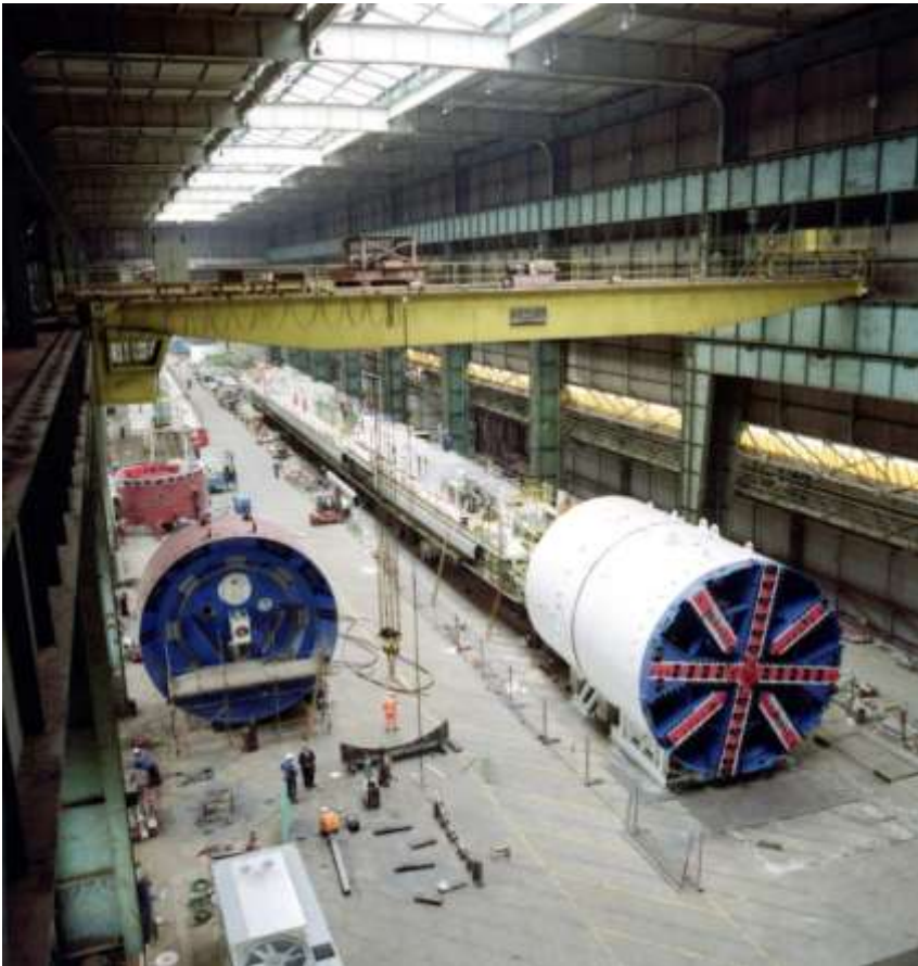
Figure 34: Photograph of a typical tunnel boring machine
