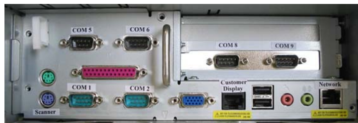
Figure 27 Epson IR 700 – showing rear connections with protective cover removed
