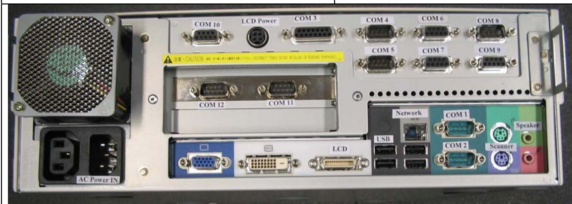
Figure 30 Fujitsu team POS 2000-M, schematic view showing ports and connections – cover removed
