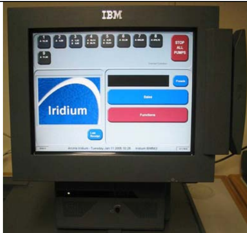
Figure 22 IBM surePOS 563, showing integrated card swipe
