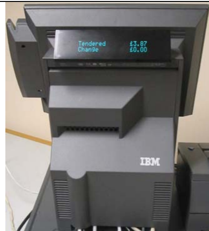
Figure 23 IBM surePOS 563, rear view showing integrated CDU
