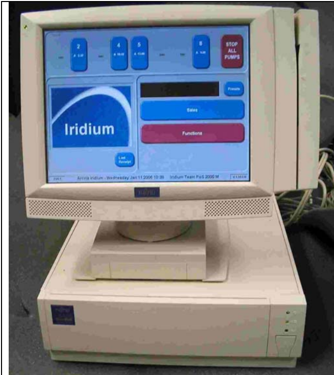
Figure 28 Fujitsu team POS 2000-M, showing integrated card swipe
