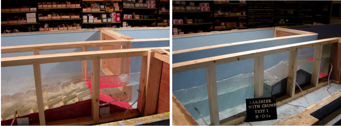
Figure K.1 Head on Larinier fishpass, 0.1 m
