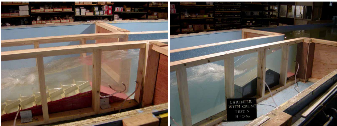
Figure K.5 Head on Larinier fishpass, 0.5 m
