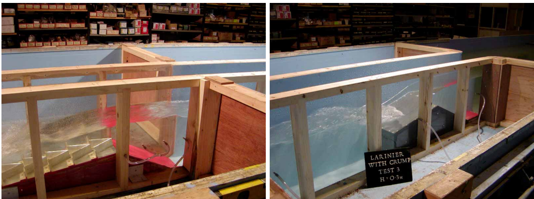
Figure K.3 Head on Larinier fishpass, 0.3 m
