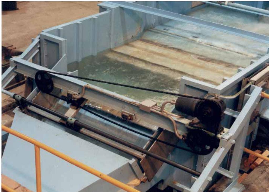
Figure F.2 Volumetric deflector gear
