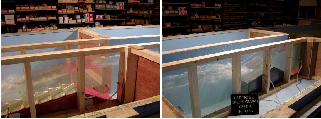
Figure K.4 Head on Larinier fishpass, 0.4 m
