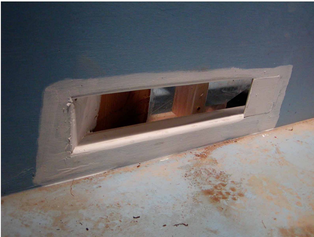
Figure L.6 Modifications to the upstream entry orifice to fishpass for Series B
