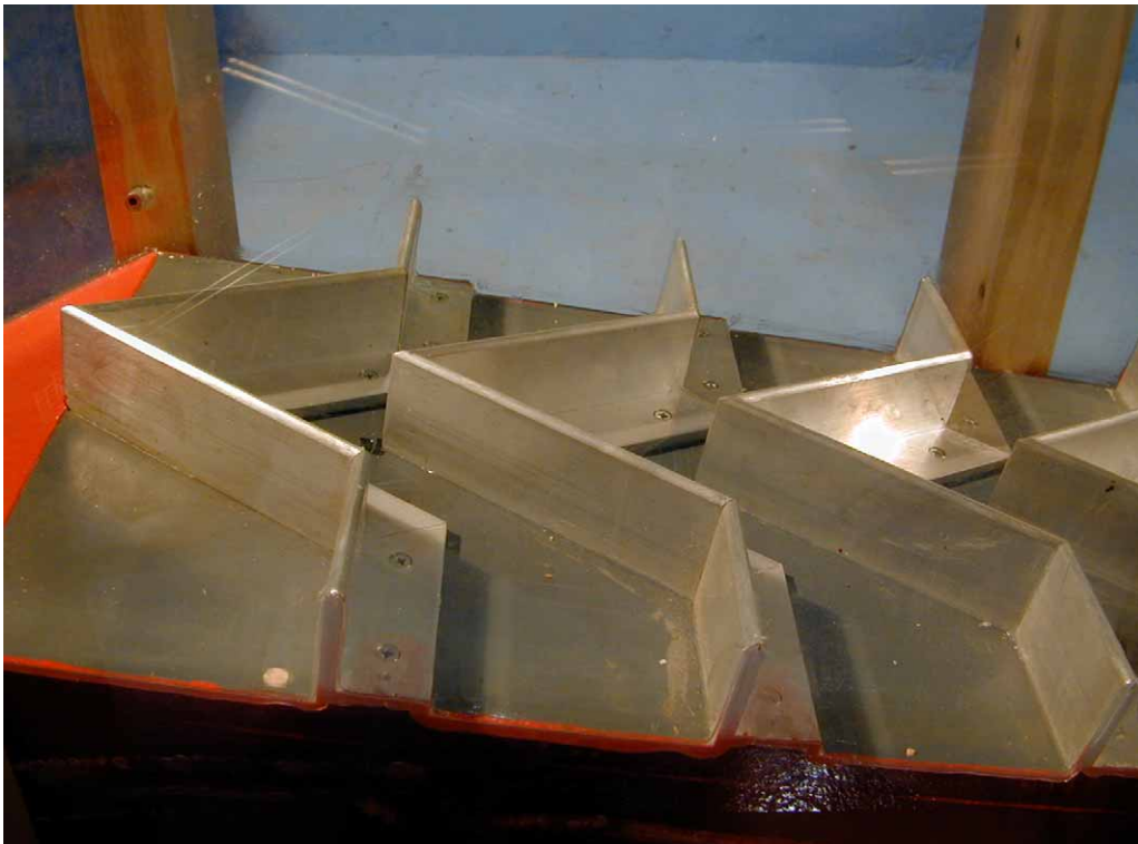
Figure I.2 First three baffles of Larinier fishpass
