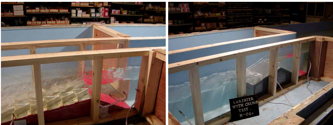
Figure K.2 Head on Larinier fishpass, 0.2 m
