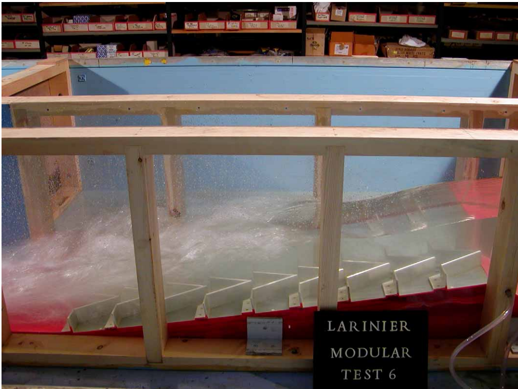
Figure I.5 Flow conditions at a head of 0.4m
