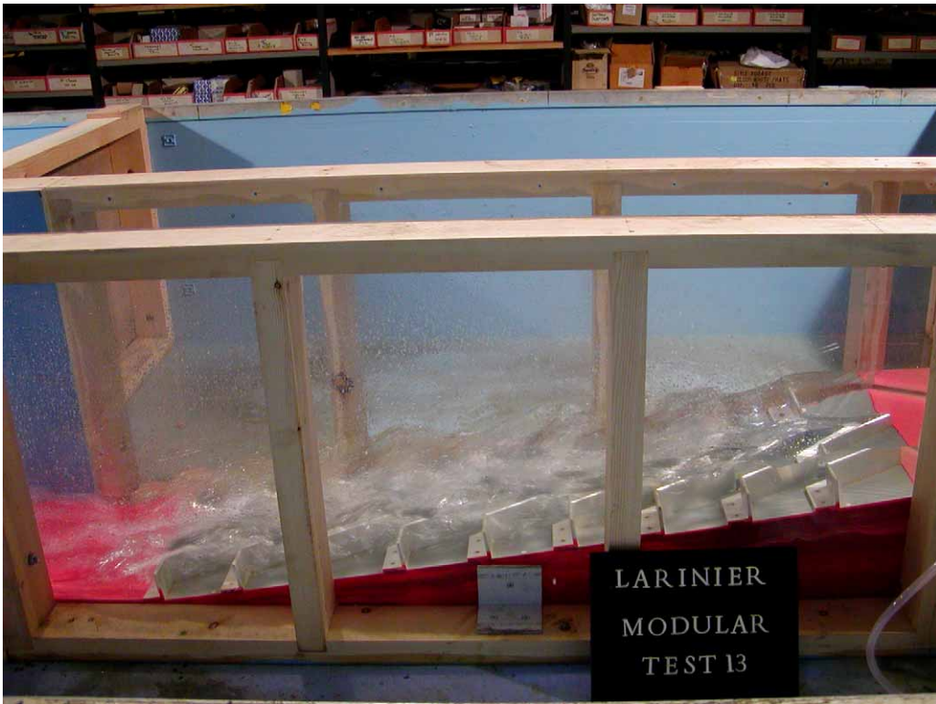
Figure I.3 Flow conditions at a head of 0.1m
