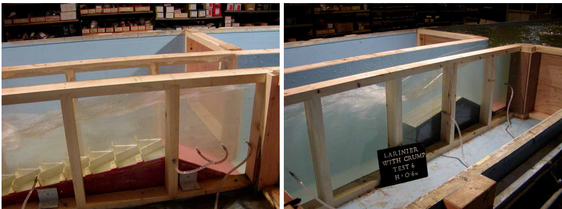
Figure K.6 Head on Larinier fishpass, 0.6 m
