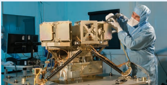
MIRI undergoing alignment testing at RAL before delivery to NASA Credit: STFC/RAL
