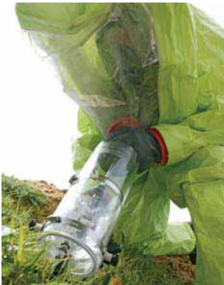
A soldier, of the Joint Nuclear, Biological & Chemical Regiment, taking an air sample from a contamination site during a simulated training exercise
