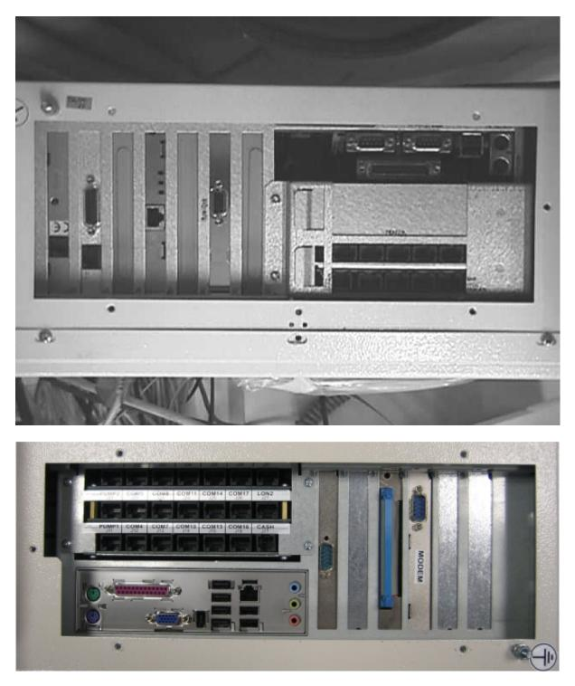
Figure 4 Passport Europe PC External Connection Ports (later version shown in lower image)
