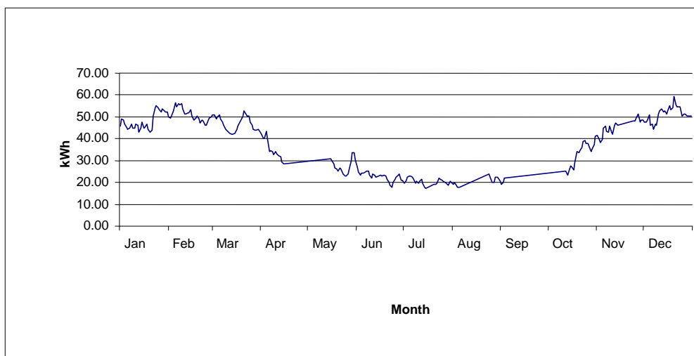
Figure 8.2 Base load electrical consumption at Kennet pumping station in 2007
