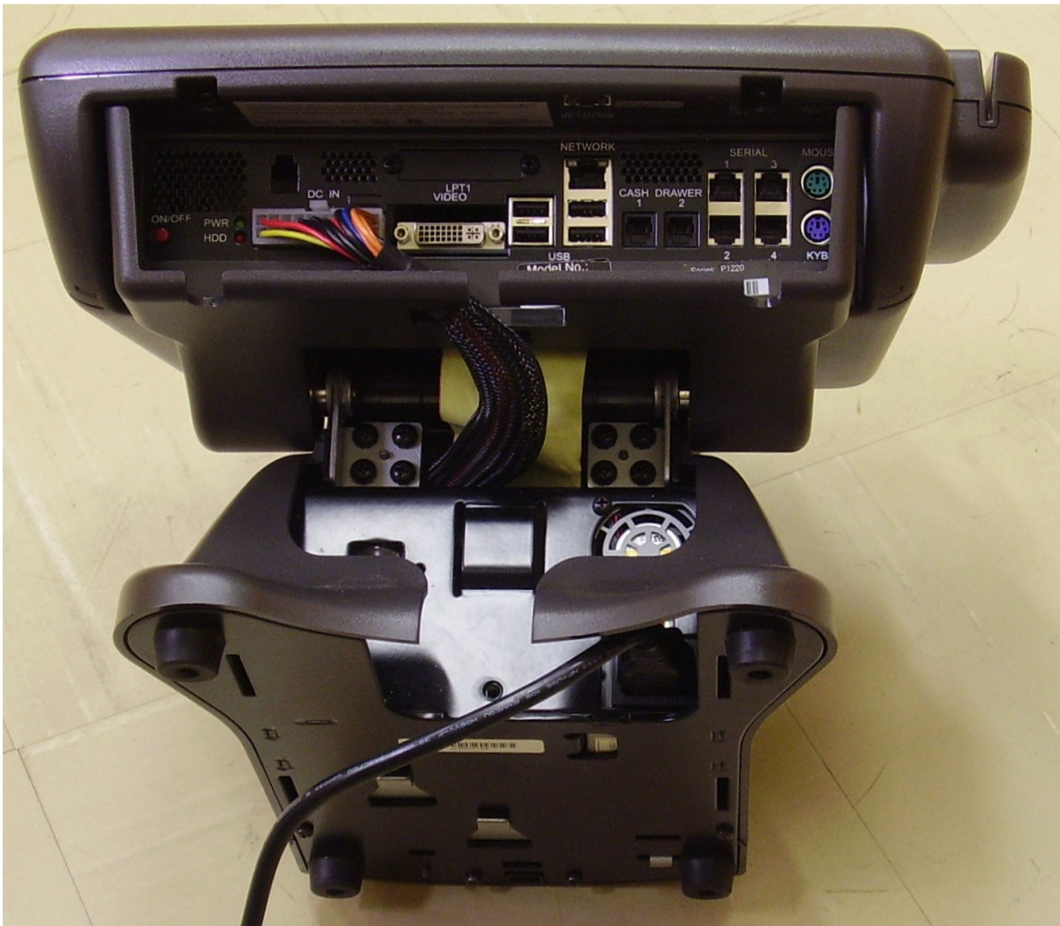
Figure 19 Port layout of P1220 with integral power supply
