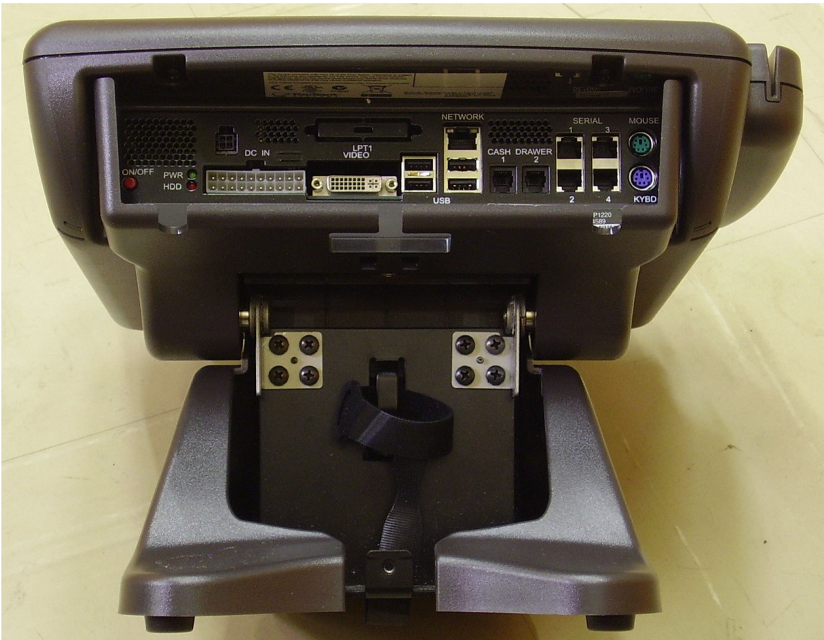
Figure 20 Port layout of P1220 with external power supply
