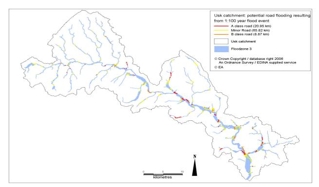
Figure 7.7: Potential road flooding resulting from a 1 in 100 year flood in the Usk catchment
