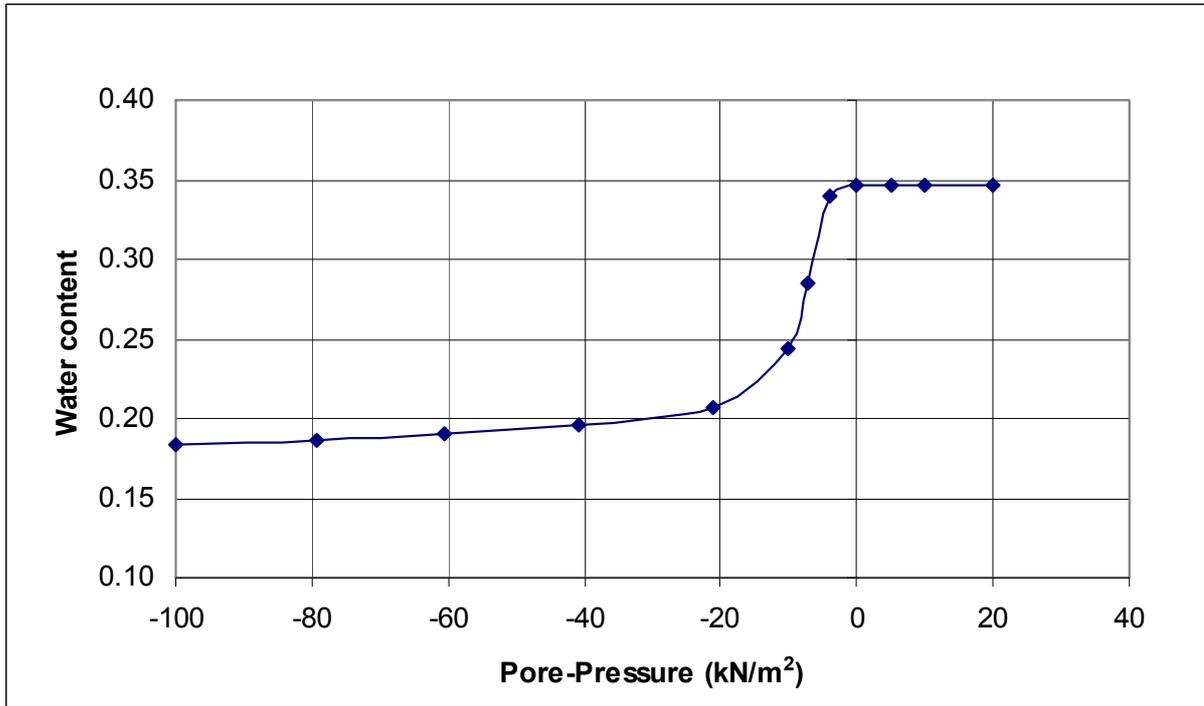
Figure A1.2 Conceptual diagram of initial water content distribution in a fully drained landfill.
