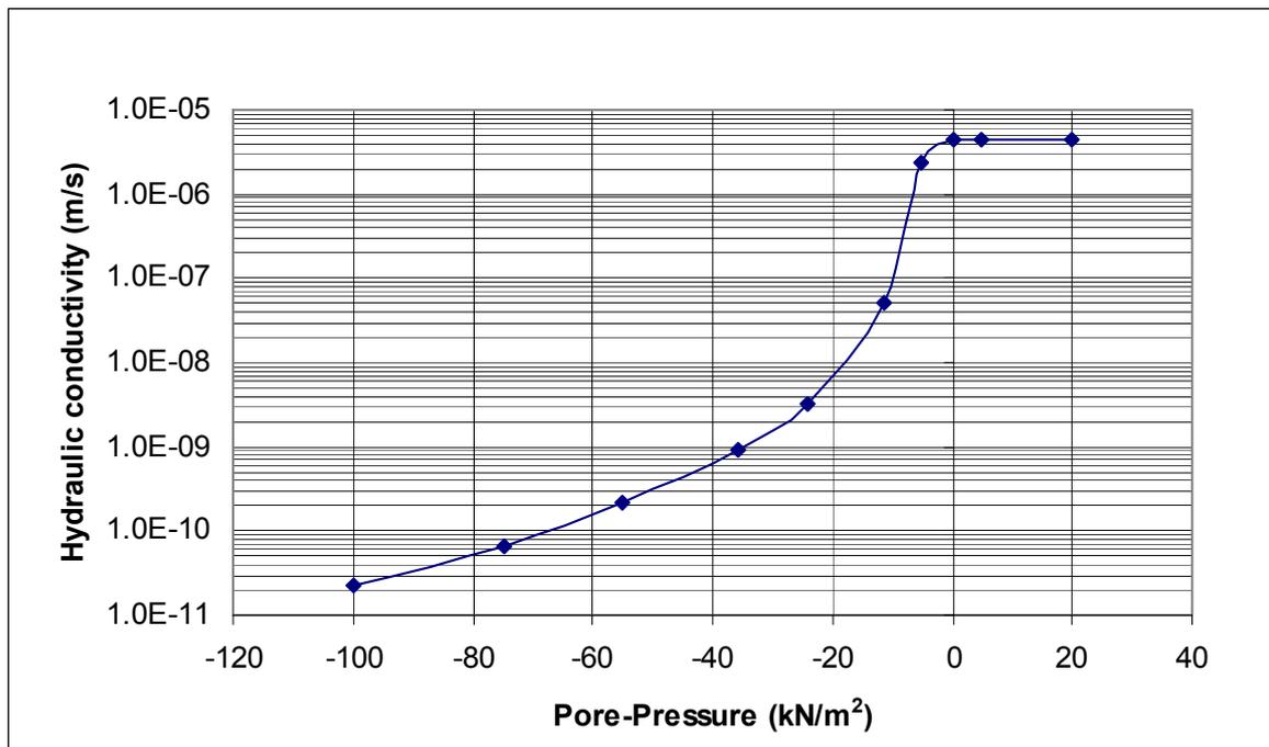
Figure A1.5 The relationship between hydraulic conductivity and water content implied by the relationships shown in Figures A1.1 and A1.4.
