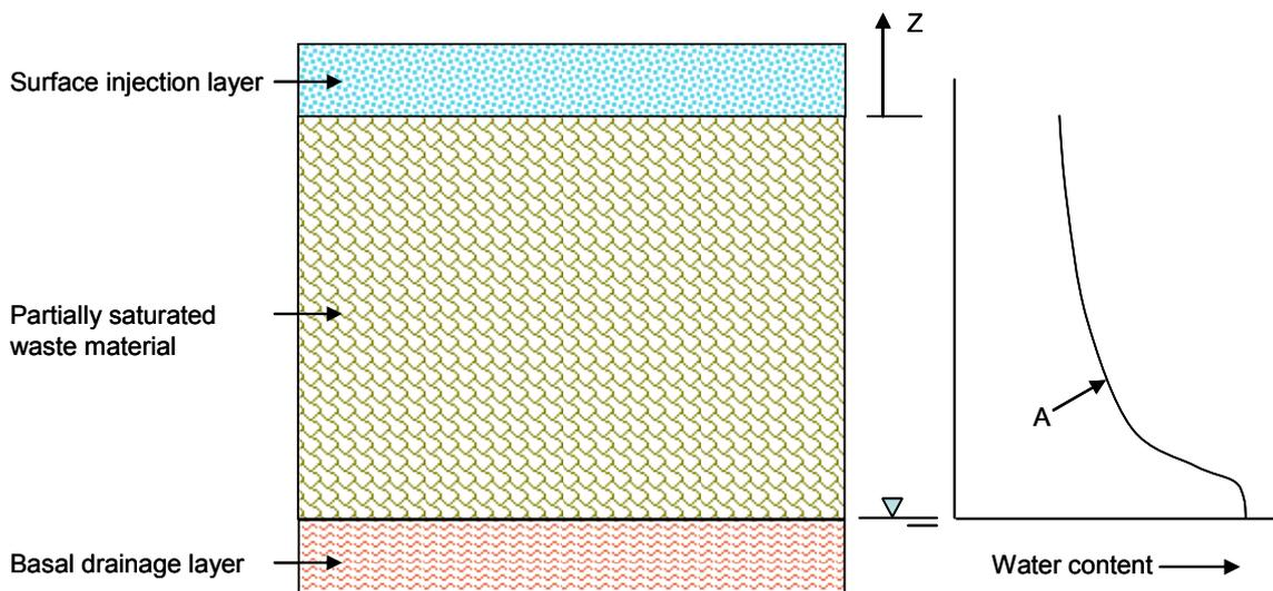
**Figure A1.3 Transient water content following start up of recirculation.**
