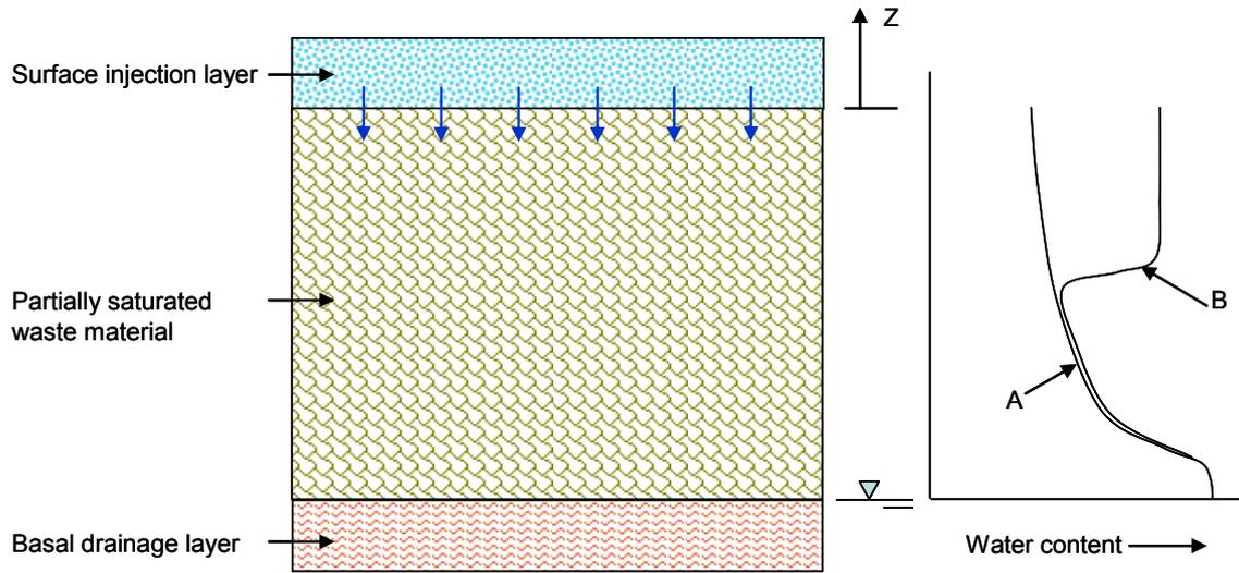
**Figure A1.4 Example of the relationship between hydraulic conductivity and pore-pressure.**
