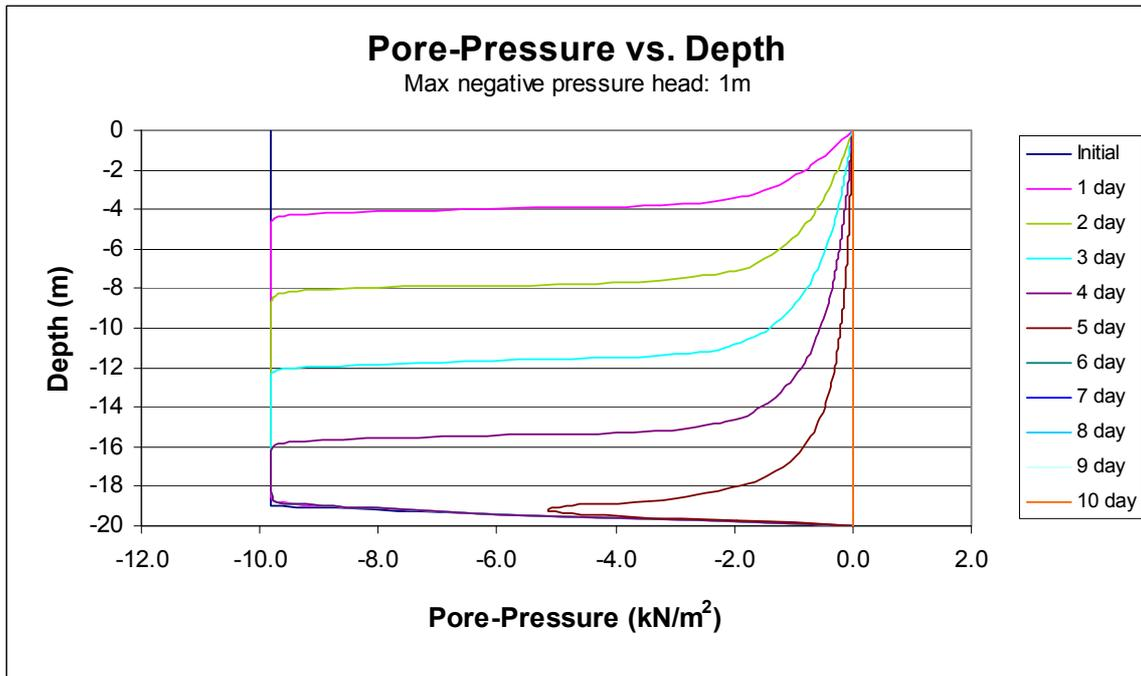
Figure A1.9 SEEP/W result showing transient of water content distribution for Case B.
