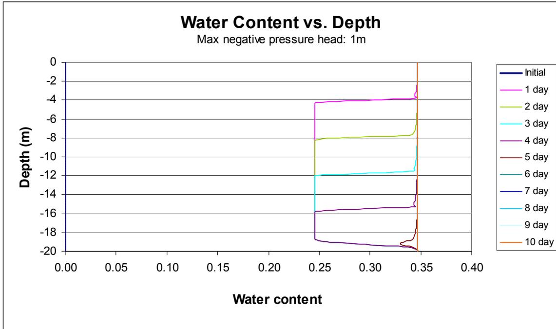
Figure A1.8 SEEP/W result showing transient of pore-pressure distribution for Case A.
