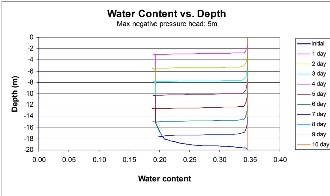
Figure A1.10 SEEP/W result showing transient of pore-pressure distribution for Case B.
