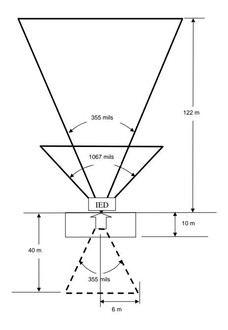
Figure 2 - Danger Areas for EOD Disruptor Weapons Injector EOD L2A1 & L3A1.
