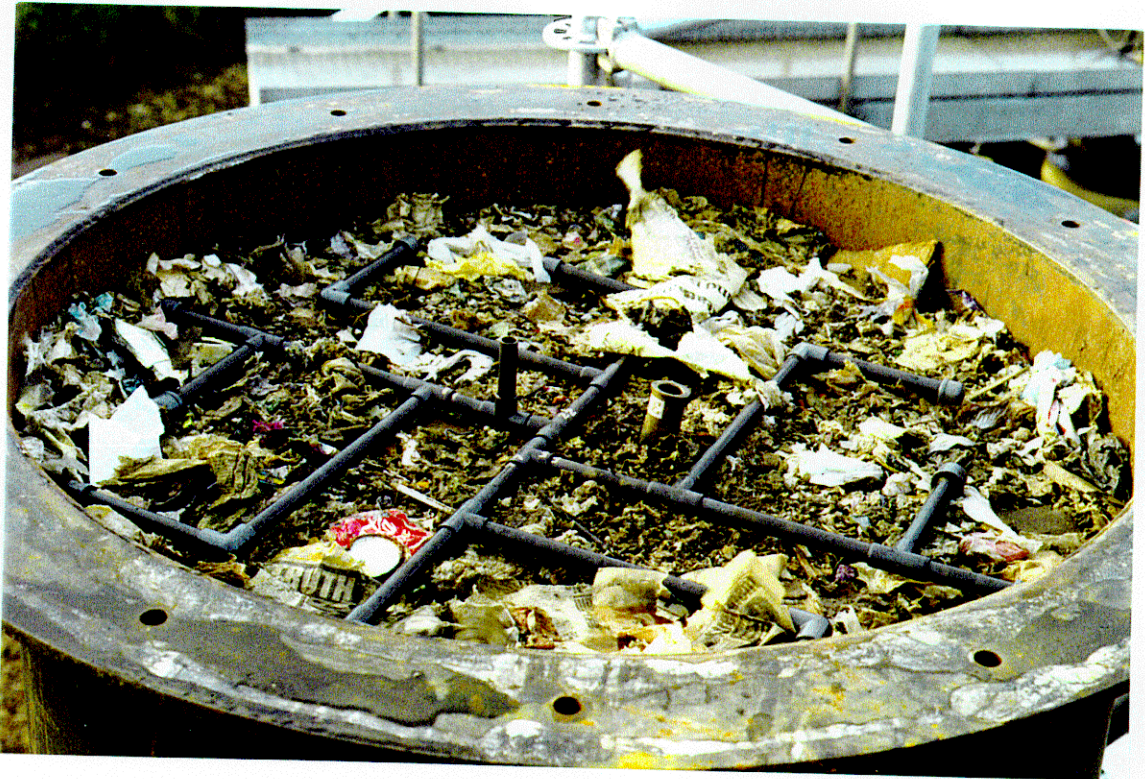
Plate 5. Young refuse batch used in this study, packed into reactor
