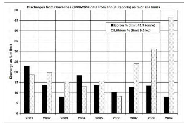
Figure A5.11 Discharges of boron and lithium from Gravelines, 2001–2009 (normalised to site limit)
