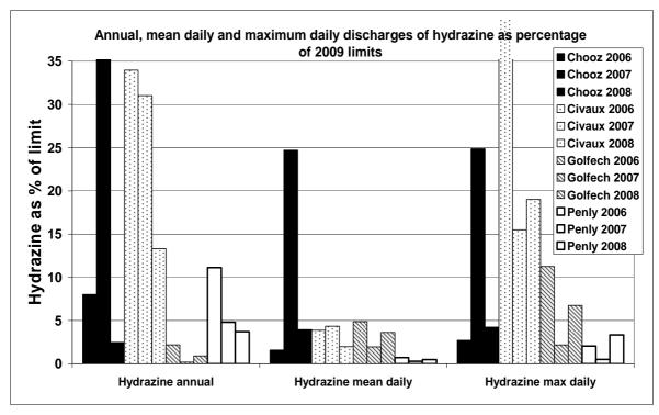
Figure A5.5 Detailed data for discharges of hydrazine
