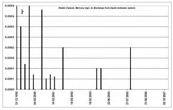
Figure A4.40 Diablo Canyon: mercury (maximum, mg/l) in discharge from the liquid radioactive waste system
