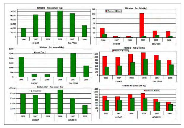
Figure A6.6 Nitrates, nitrites and sodium in effluents associated with biocide treatment, Chooz and Golfech
