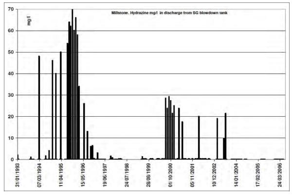
Figure A4.52 Millstone: hydrazine (maximum, mg/l) in discharge from steam generator blowdown tank
