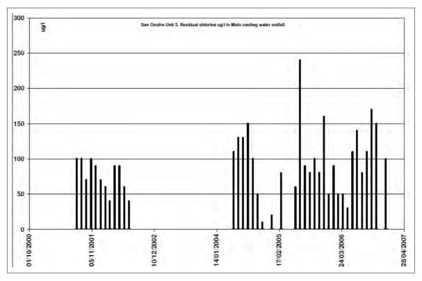
Figure A4.31 San Onofre Unit 3: total residual chlorine (maximum,  $\mu$ g/l) in main cooling water discharge
