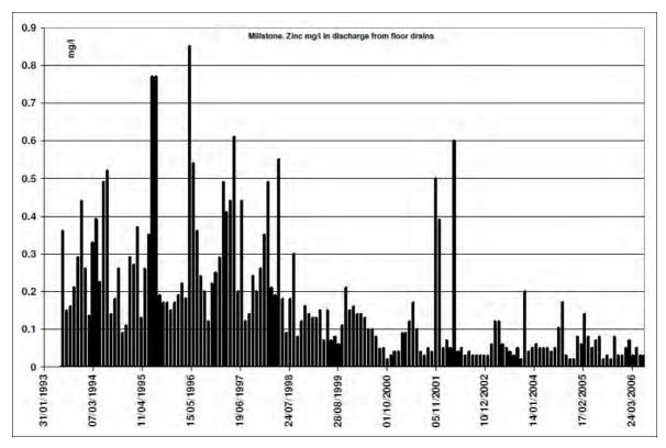
Figure A4.51 Millstone: zinc (maximum, mg/l) in discharge from floor drains
