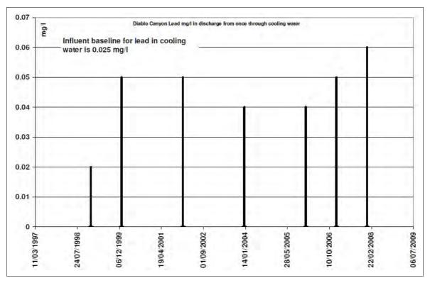
Figure A4.36 Diablo Canyon: lead (maximum, mg/l) in once through cooling water discharge
