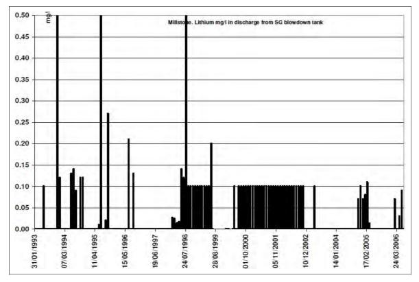
Figure A4.55 Millstone: lithium (maximum, mg/l) in discharge from steam generator blowdown tank
