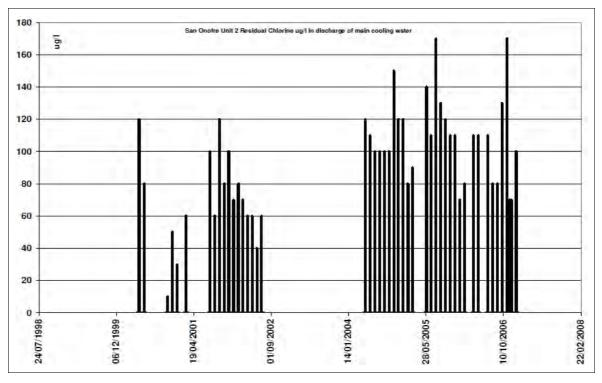
Figure A4.28 San Onofre Unit 2: total residual chlorine (maximum, µg/l) in discharge of main cooling water
