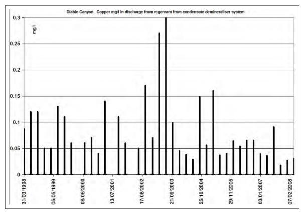
Figure A4.43 Diablo Canyon: copper (maximum, mg/l) in discharge from regeneration of the condensate polishing plant
