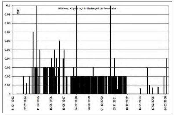
Figure A4.50 Millstone: copper (maximum, mg/l) in discharge from floor drains
