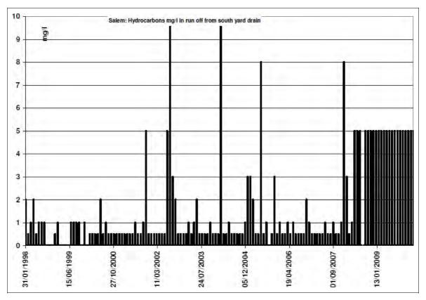
Figure A4.26 Salem: total hydrocarbons (maximum, mg/l) in discharge from yard drains
