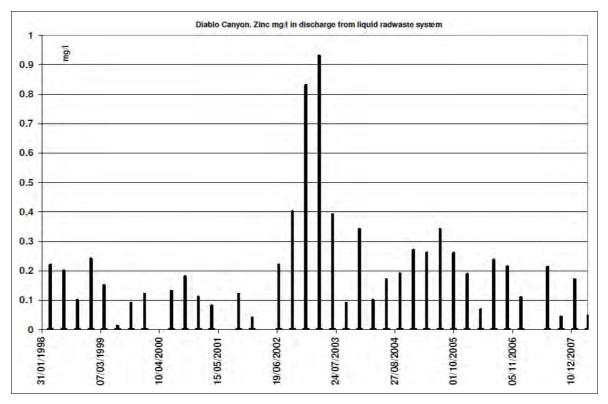
Figure A4.41 Diablo Canyon: zinc (maximum, mg/l) in discharge from the liquid waste system
