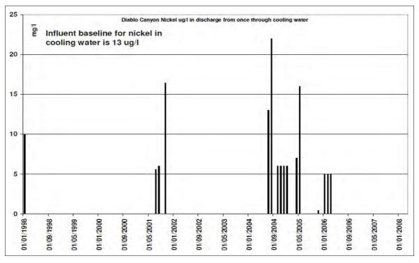
Figure A4.37 Diablo Canyon: nickel (maximum, µg/l) in once through cooling water discharge
