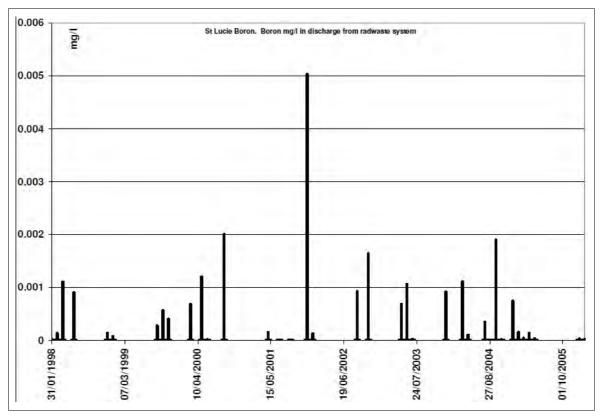
Figure A4.57 St Lucie: boron (maximum, mg/l) in discharge from radioactive waste system
