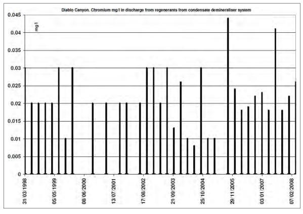
Figure A4.42 Diablo Canyon: chromium (maximum, mg/l) in discharge from regeneration of the condensate polishing plant
