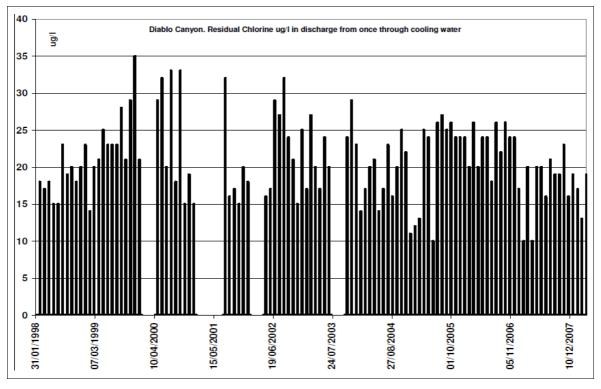
Figure A4.33 Diablo Canyon: chlorine (mean, µg/l) in once through cooling water discharge
