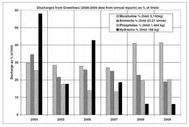
Figure A5.12 Discharges of morpholine, ammonia, phosphates and hydrazine from Gravelines 2004–2009 (normalised to site limits)
