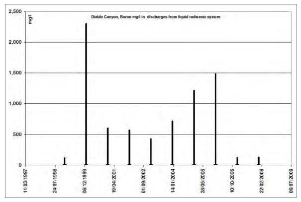
Figure A4.38 Diablo Canyon: boron (maximum, mg/l) in discharge from the liquid radioactive waste system
