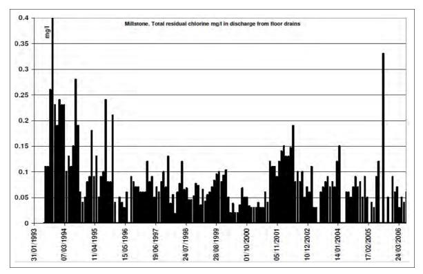
Figure A4.49 Millstone: residual chlorine (maximum, mg/l) in discharge from floor drains
