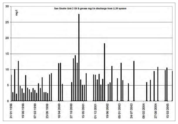
Figure A4.30 San Onofre Unit 2: oil and grease (maximum, mg/l) in discharge of low level waste water
