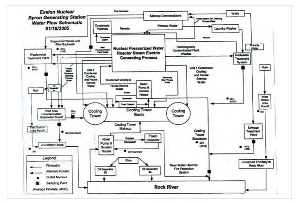
Figure A3.2 Byron water flow and balance diagram (by permission of Byron Plant)
