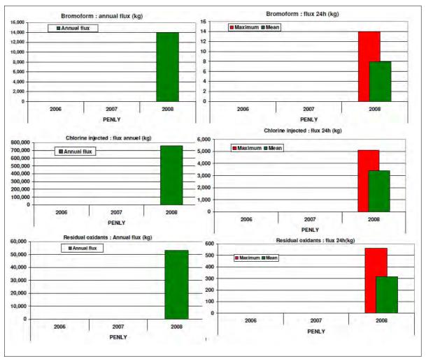
Figure A6.7 Bromoform, injected chlorine and residual oxidants in effluents associated with electrochlorination (Penly only)
