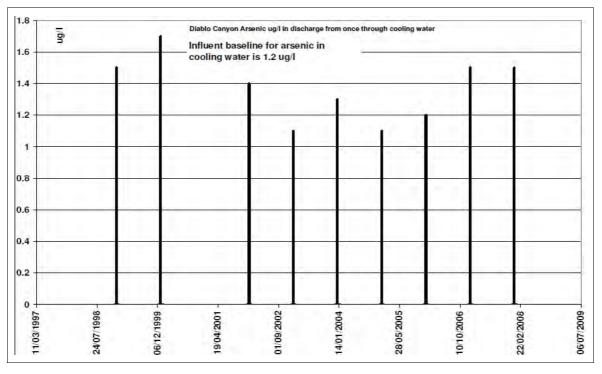
Figure A4.34 Diablo Canyon: arsenic (maximum, µg/l) in once through cooling water discharge
