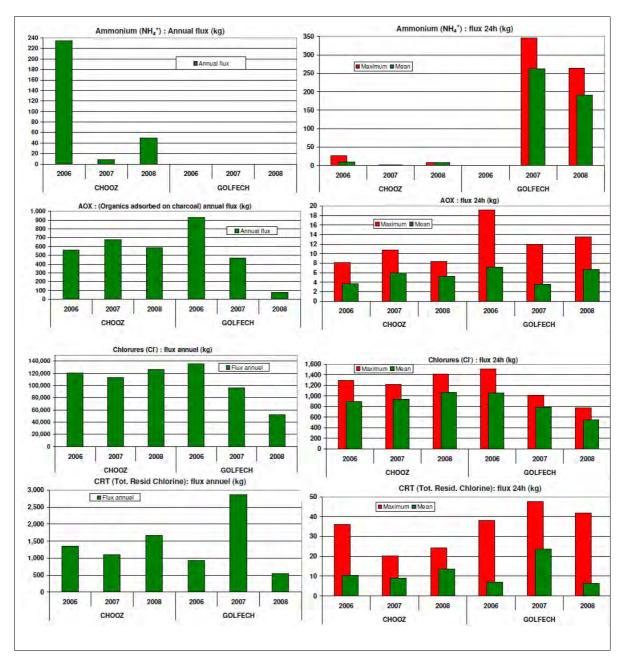
Figure A6.5 Ammonium, AOX, chlorides and total residual chlorine in discharges associated with biocide treatment at Chooz and Golfech
