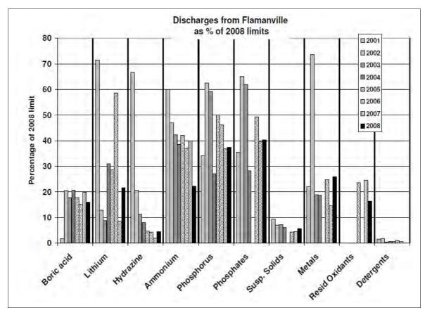
Figure A5.9 Discharge data for Flamanville plotted by parameter (normalised to site limit)
