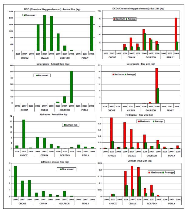
Figure A6.2 Chemical oxygen demand, detergents, hydrazine and lithium associated with liquid radioactive effluents from the nuclear island and turbine hall discharge (KER-SEK)
