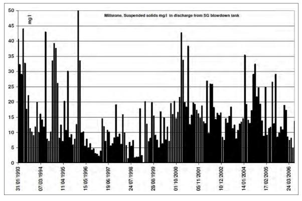
Figure A4.54 Millstone: solids (maximum, mg/l) in discharge from steam generator blowdown tank
