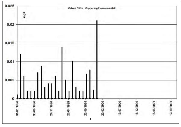
Figure A4.60 Calvert Cliffs: copper (maximum, mg/l) in main cooling water discharge
