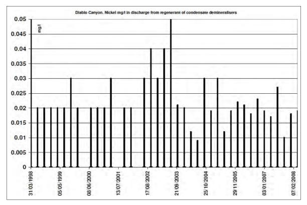
Figure A4.45 Diablo Canyon: nickel (maximum, mg/l) in discharge from regeneration of the condensate polishing plant
