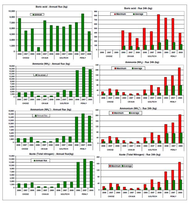
Figure A6.1 Boric acid, ammonia, ammonium and total nitrogen associated with liquid radioactive effluents from the nuclear island and turbine hall discharge (KER-SEK)
