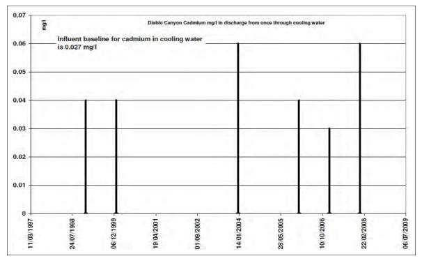
Figure A4.35 Diablo Canyon: cadmium (maximum, mg/l) in once through cooling water discharge
