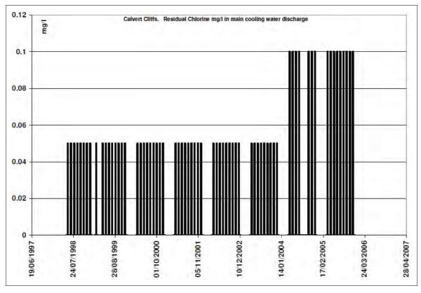
Figure A4.59 Calvert Cliffs: residual chlorine (maximum, mg/l) in discharge from main cooling water
