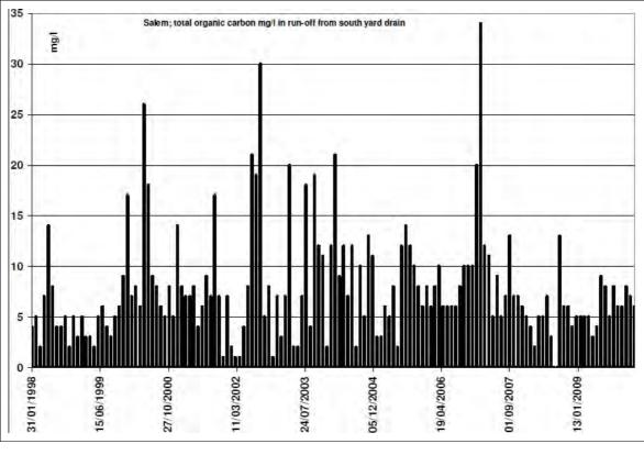
Figure A4.27 Salem: total organic carbon (maximum, mg/l) in discharge from yard drains
