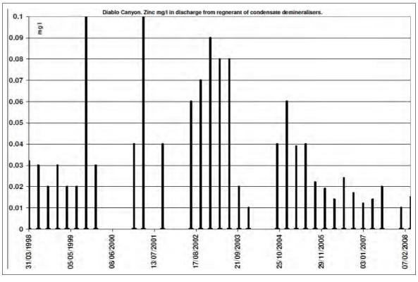
Figure A4.46 Diablo Canyon: zinc (maximum, mg/l) in discharge from regeneration of the condensate polishing plant
