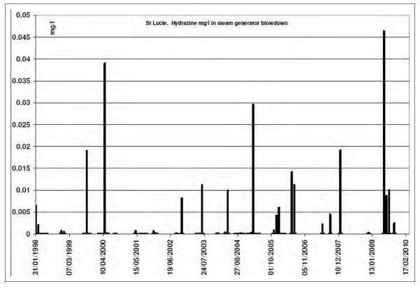
Figure A4.58 St Lucie: hydrazine (maximum, mg/l) in steam generator blowdown
