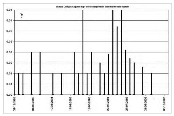
Figure A4.39 Diablo Canyon: copper(maximum, mg/l) in discharge from the liquid radioactive waste system
