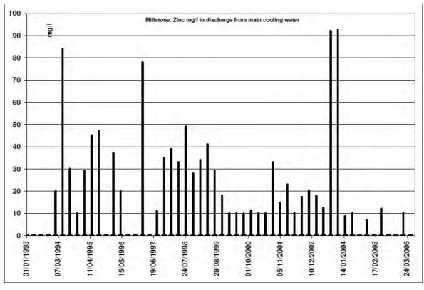
Figure A4.48 Millstone: zinc (maximum, mg/l) in discharge from main cooling water system
