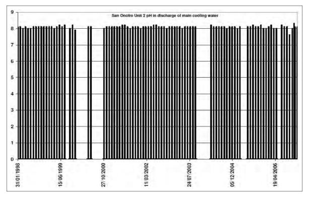
Figure A4.29 San Onofre Unit 2: pH (maximum) of discharge of main cooling water
