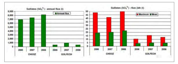
Figure A6.10 Sulphate discharges due to anti-scale treatments at Chooz and Golfech
