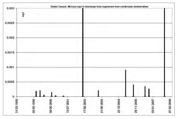
Figure A4.44 Diablo Canyon: mercury (maximum, mg/l) in discharge from regeneration of the condensate polishing plant
