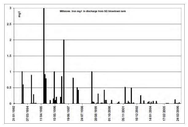
Figure A4.53 Millstone: iron (maximum, mg/l) in discharge from steam generator blowdown tank
