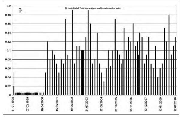
Figure A4.56 St Lucie: total residual oxidants (mean, mg/l) in discharge of main cooling water
