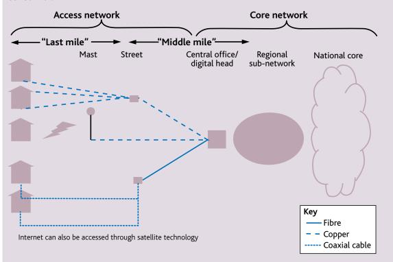
The access layer of the network is generally the line between the exchange and the premises. Next generation fixed networks tend to replace part or all of the copper connection between those two points. Typically, NGA networks (Next Generation Access – high speed broadband access to the home, usually using fibre optic technology) tend to be 'fibre to the cabinet' (with a copper connection from the cabinet to the premises); or 'fibre to the home'.
