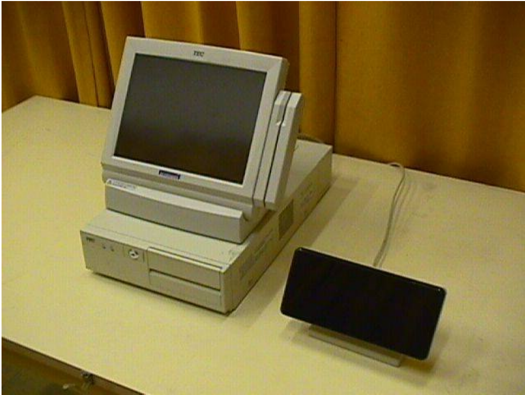
Figure 8 Toshiba TEC 5600 point of sale
