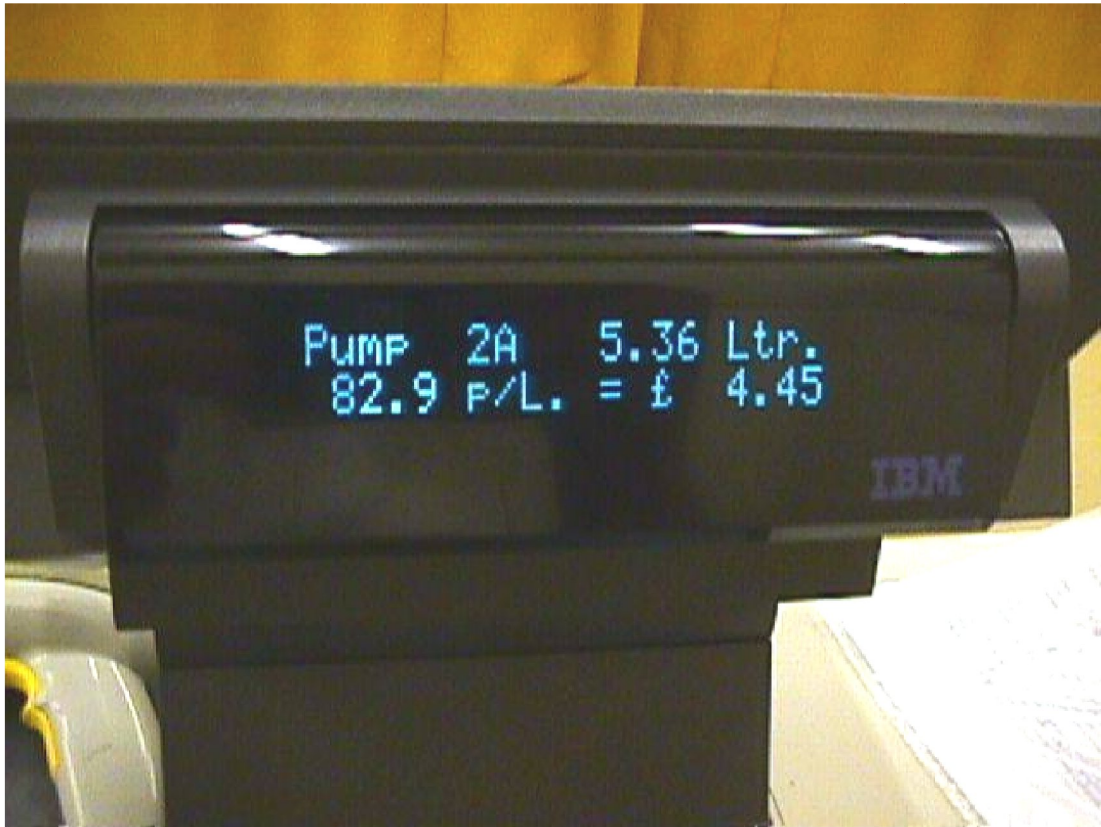
Figure 3 IBM SurePos integrated CDU
