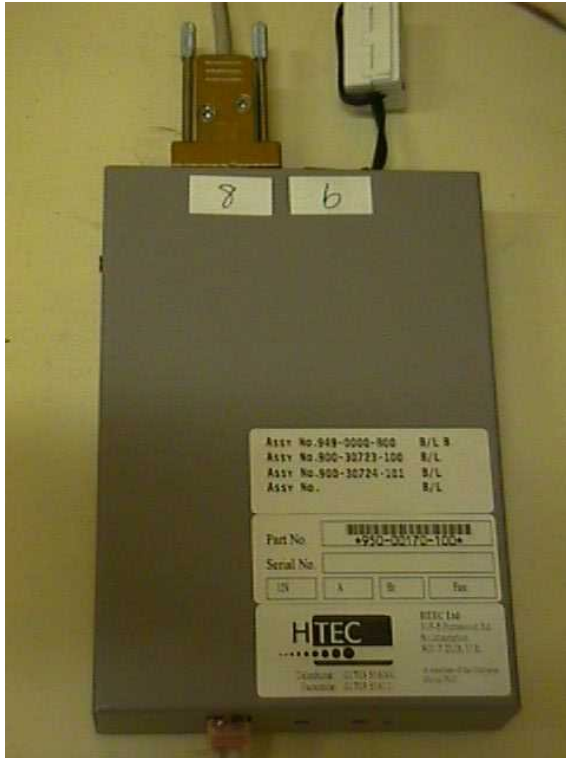
Figure 12 RS232 / LON interface unit
