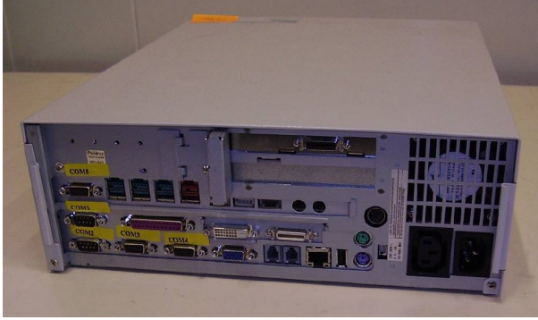
Figure 39 Port layout of ST-7000
