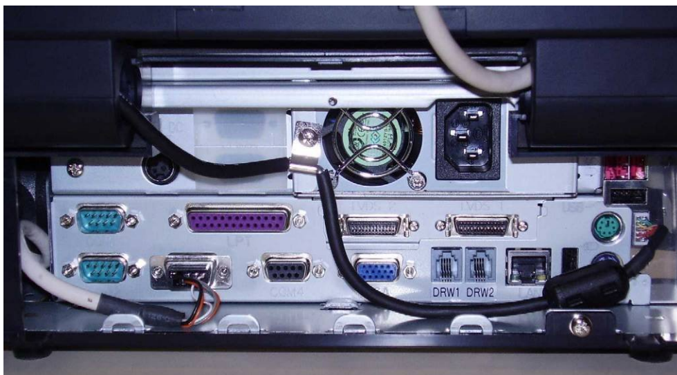
Figure 37 Port layout of ST-71 terminal
