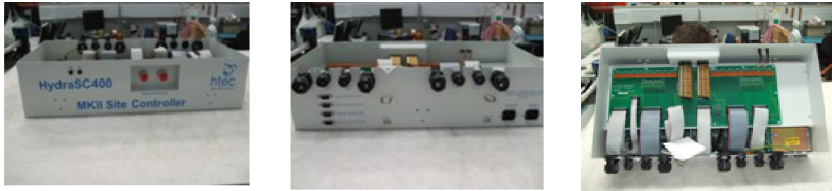
Figure 52 HTEC Hydra SC400 MkII site controller, part number 950-00251-100 (Resilient) also termed EC resilient site controller
