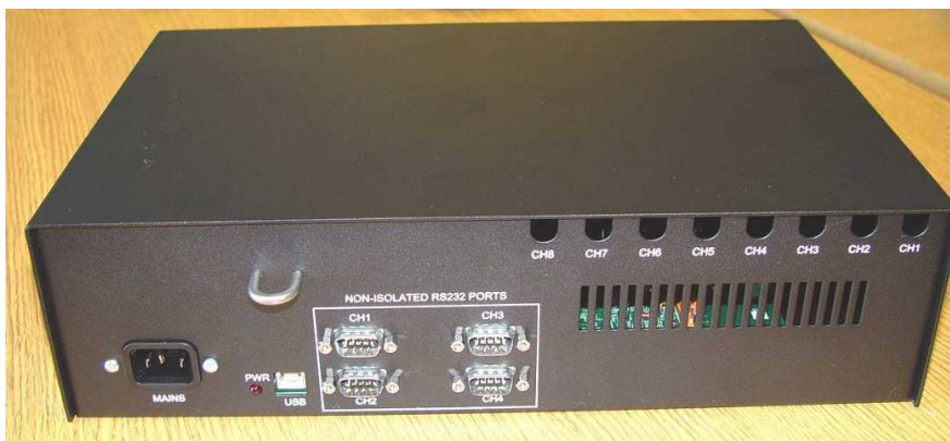
Figure 15 HTEC pump interface 950-00210-100: rear view showing connections
