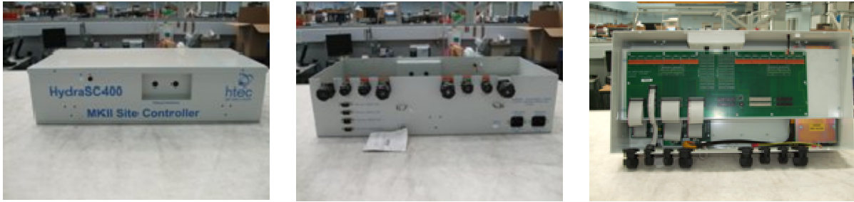
Figure 51 Alternative HTEC pump interface unit, part number 950-00251-101, also termed side A only controller
