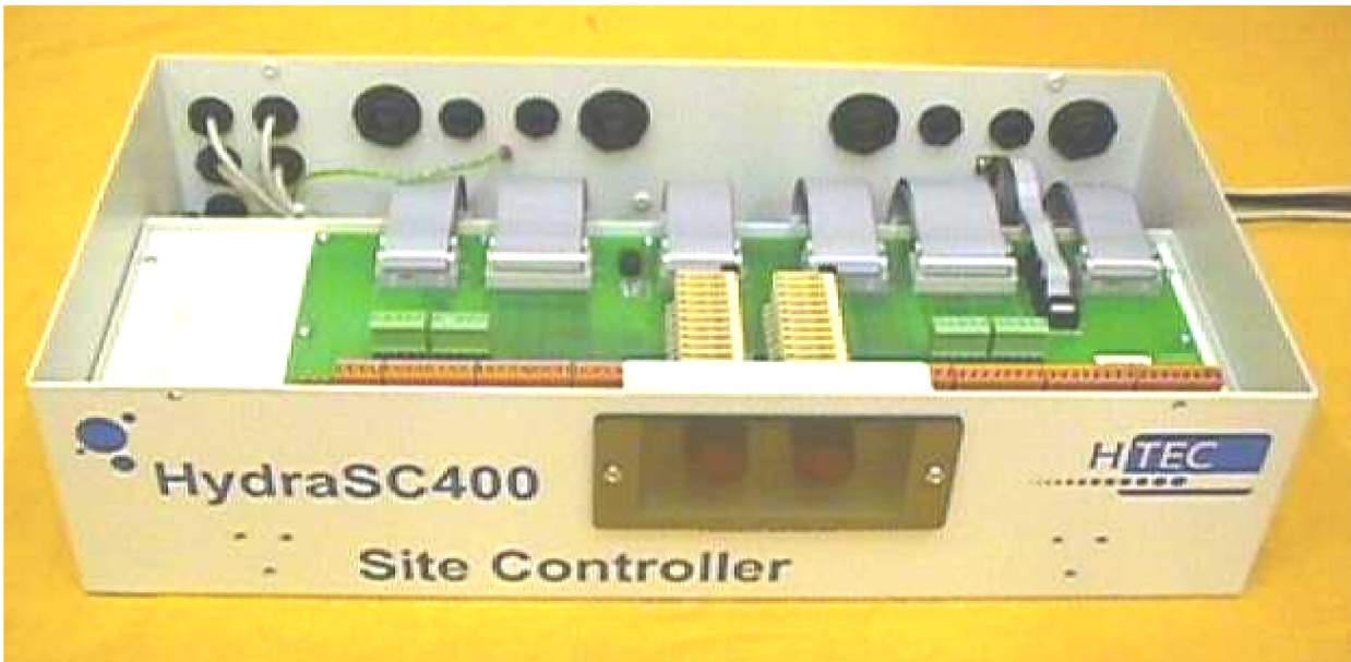
Figure 19 HTEC Hydra SC400 site controller - part number 950-00214-100: front view showing fault condition changeover switches
