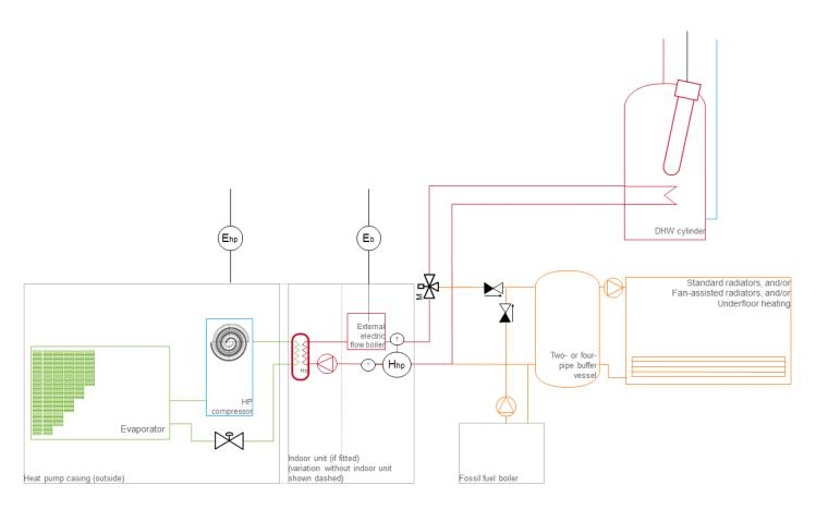
Figure 11: Split-system air-source heat pump with metering option 2: 1 heat meter (integrated), 2 electricity meters
