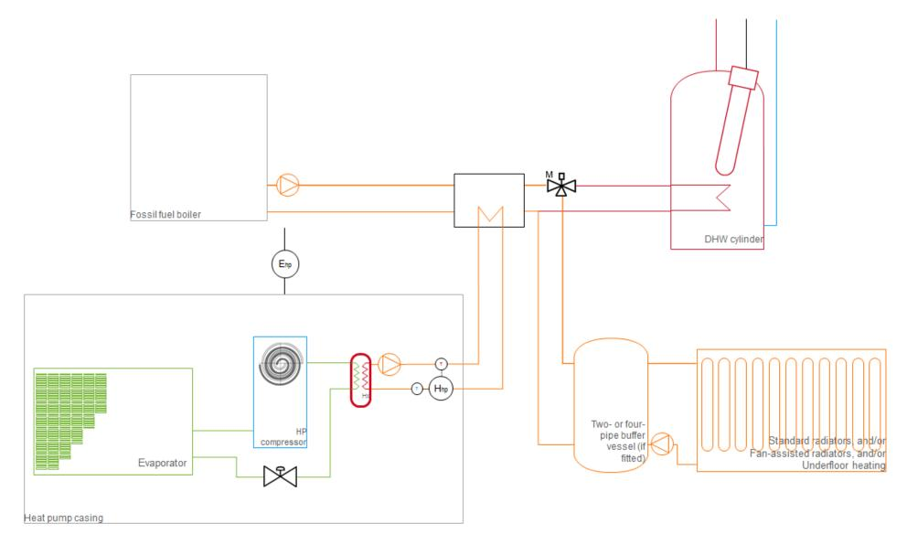
Figure 5: Air-source heat pump with back-up fossil fuel boiler showing metering option 2: 1 heat meter (integrated) and 1 electricity meter
