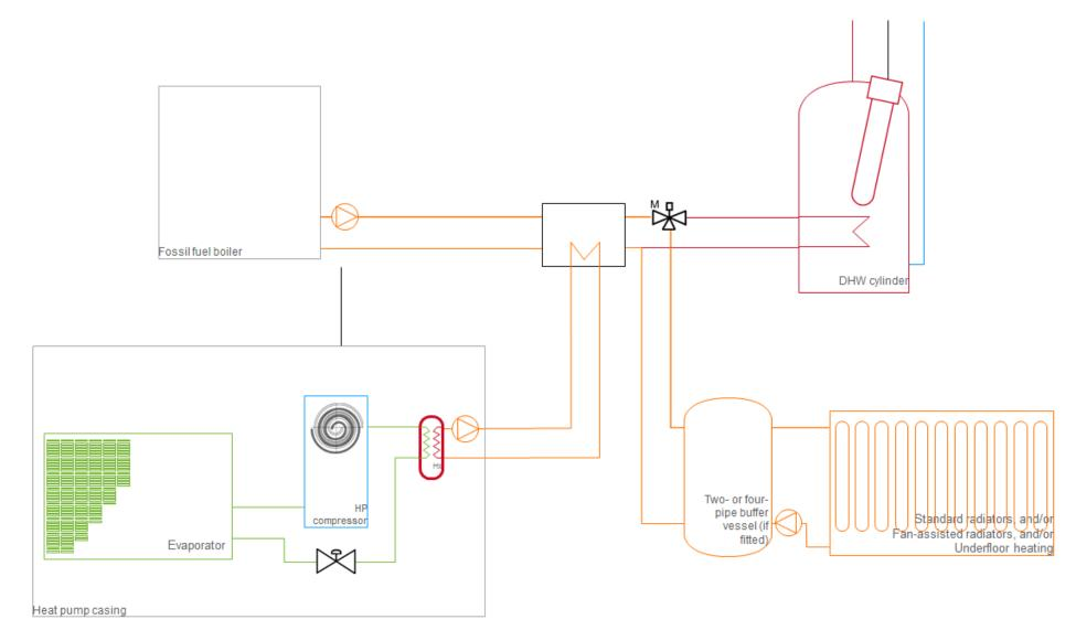
Figure 3: Air-source heat pump with back-up fossil fuel boiler
