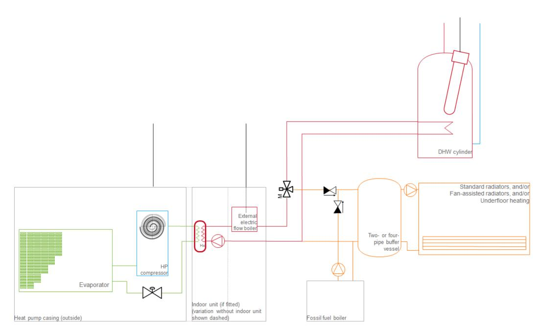
Figure 9: Split-system air-source heat pump providing space heating and hot water
