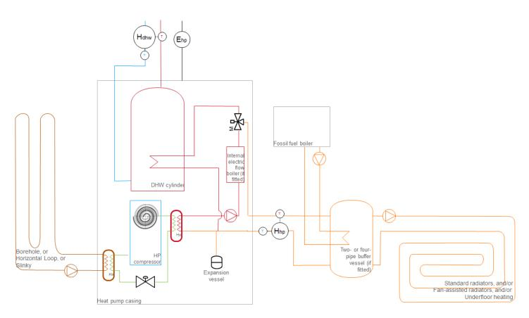
Figure 7: Ground-source heat pump with integrated domestic hot water cylinder and metering option 1: 2 heat meters, 1 electricity meter
