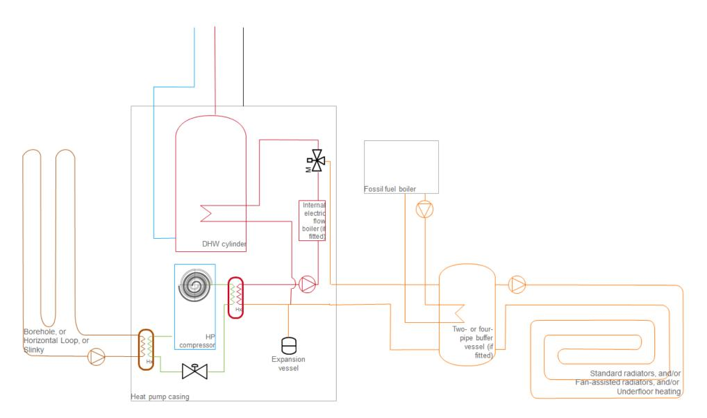
Figure 6: Ground-source heat pump with integrated domestic hot water cylinder
