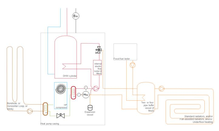
Figure 8: Ground-source heat pump with integrated domestic hot water cylinder and metering option 2: 1 heat meter (integrated), 1 electricity meter
