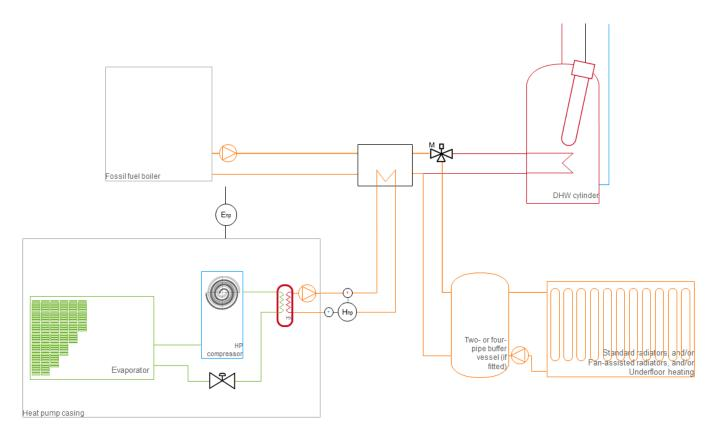
Figure 4: Air-source heat pump with back-up fossil fuel boiler showing metering option 1: 1 heat meter and 1 electricity meter
