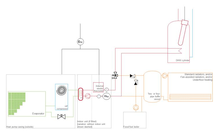
Figure 12: Split-system air-source heat pump with metering option 3: 1 heat meter (integrated), 1 electricity meter
