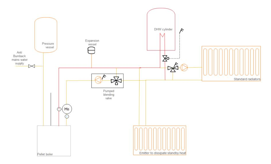
Figure 2: Pellet biomass boiler with metering option 1: 1 heat meter
