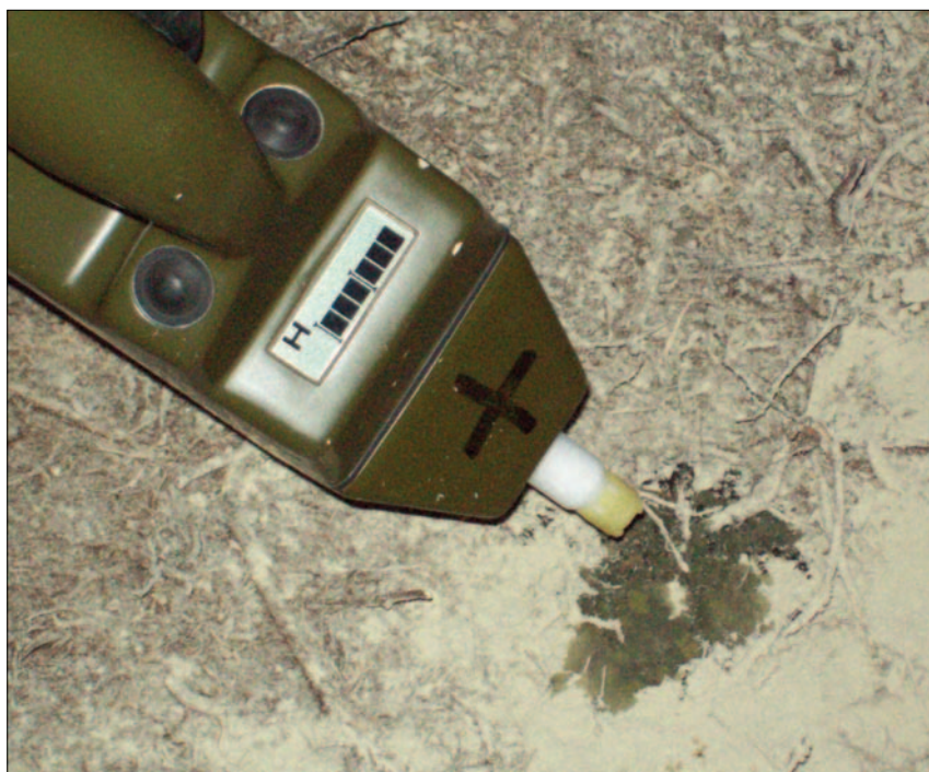
Figure 1: Field monitor for sulphur mustard. Reproduced with permission from Defence Science and Technology Lab (DSTL).
