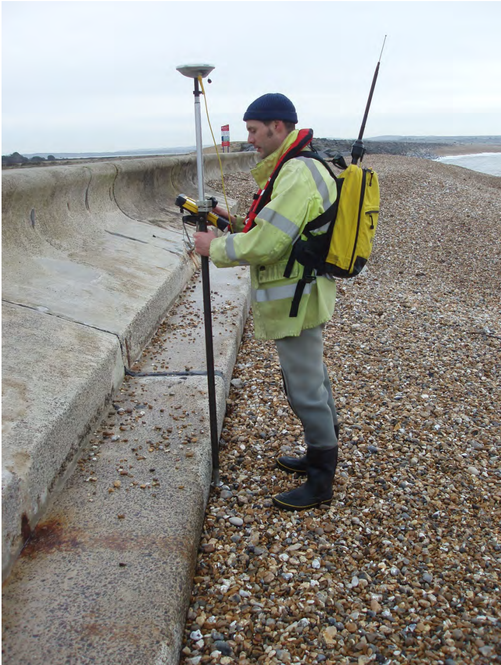
Figure 3.12 Beach survey using global positioning equipment (courtesy Channel Coastal Observatory)
