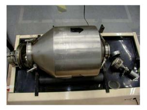
Dustiness drum -Estimation of potential for release of bioaerosols from compost material
