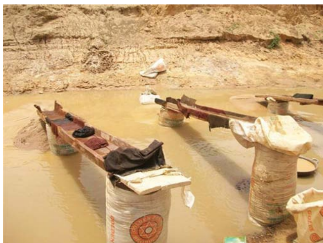
Figure 2: Pulverised rock is sluiced in a community pond to float off lighter particles (courtesy: World Health Organization)
