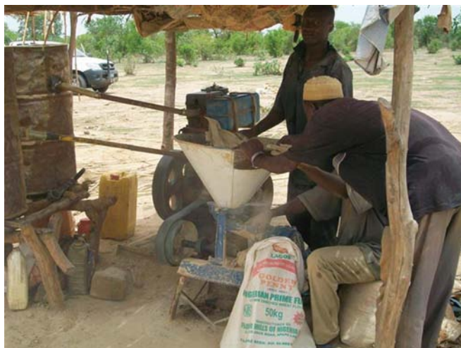
Figure 1: Lead-rich ore being ground into a fine powder before being further treated to extract gold (courtesy: World Health Organization)
