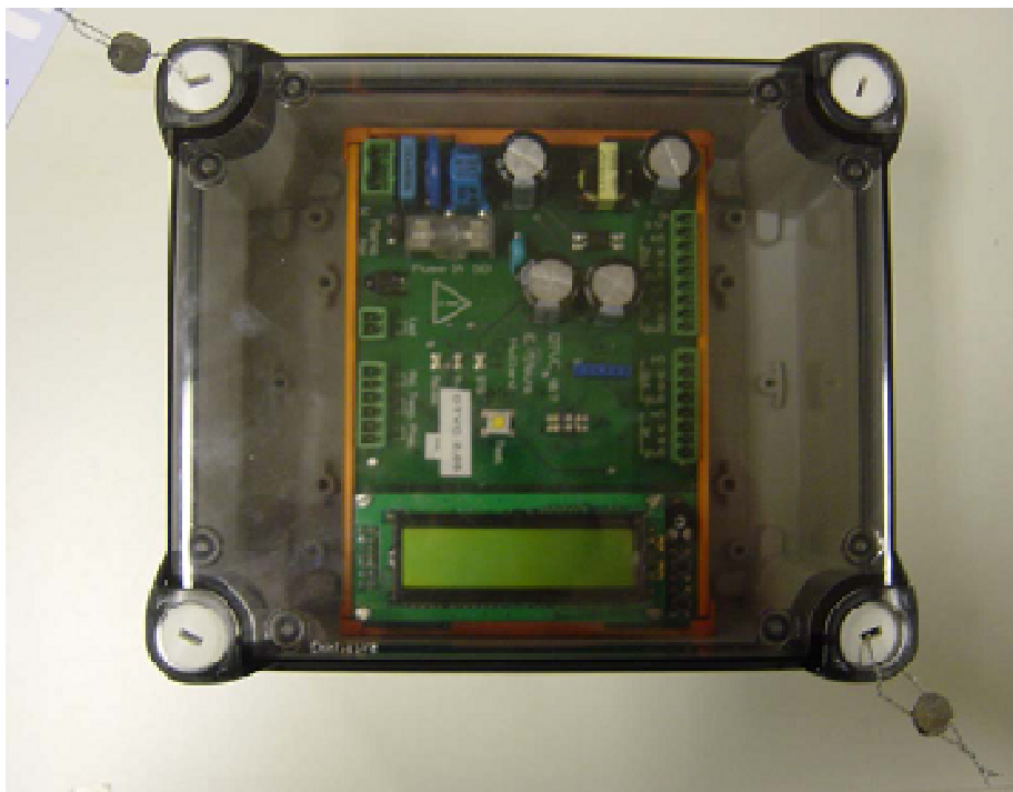
Figure 27 TVC unit sealing arrangement
