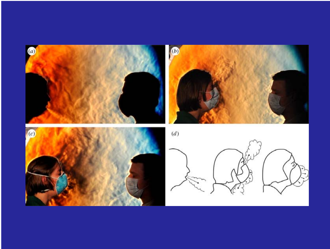
Figure 8; reproduced from (93): Schlieren images of two volunteers facing one another. The subject on the right is masked as a precaution. The volunteer on the left coughs in the direction of the other subject first without wearing a mask (a) (the cough plume can be seen directed downwards at roughly a 30° angle), then while wearing a standard surgical mask (b), and finally while wearing an N95 mask (c). The different behaviours of these coughs are sketched in (d).
