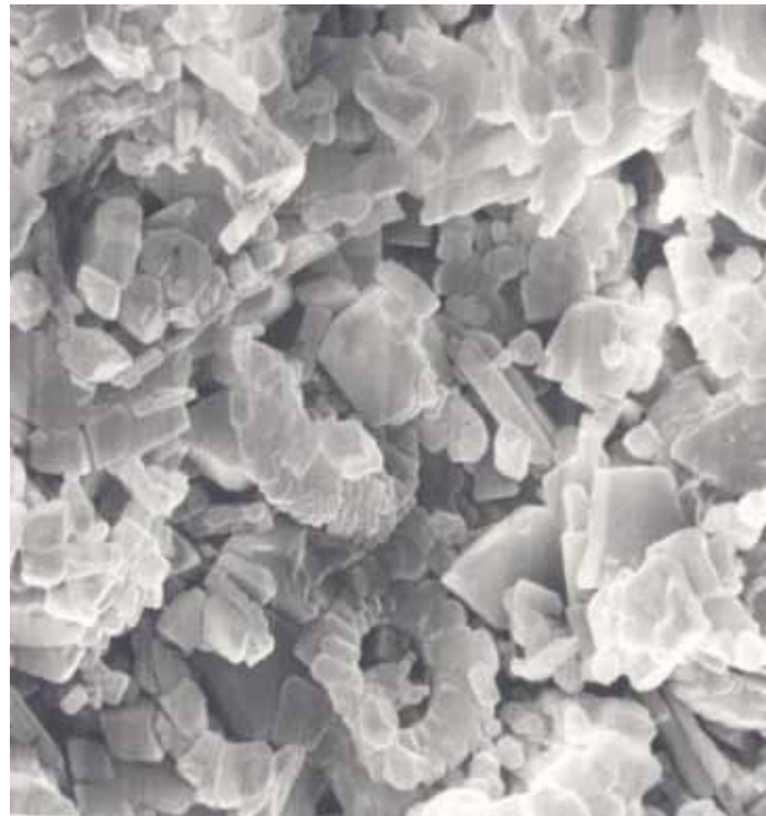
Figure 3.5 SEM photomicrograph of the Chalk showing round coccolithic fragments and calcite platelets (Field of view approximately 5 \mu\text{m} ).
