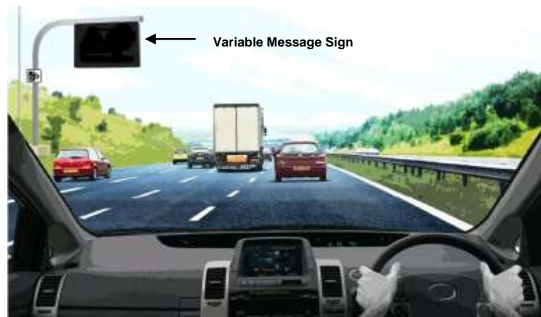
Figure 4B: Illustrative M5 Junction 4A to 6 Smart Motorway All lane Running scheme section operating in normal motorway conditions with a blank verge mounted variable message sign
