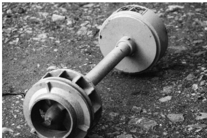
Figure 5.4 Battery-charging propeller turbine, manufactured in Vietnam
