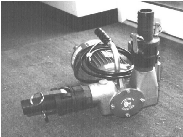
Figure 3.3 FI ITT Jabsco direct driven rotary flexible impeller pump
