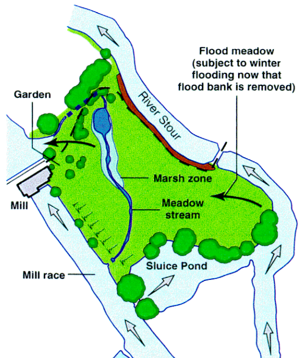
Plan of site after work completed
