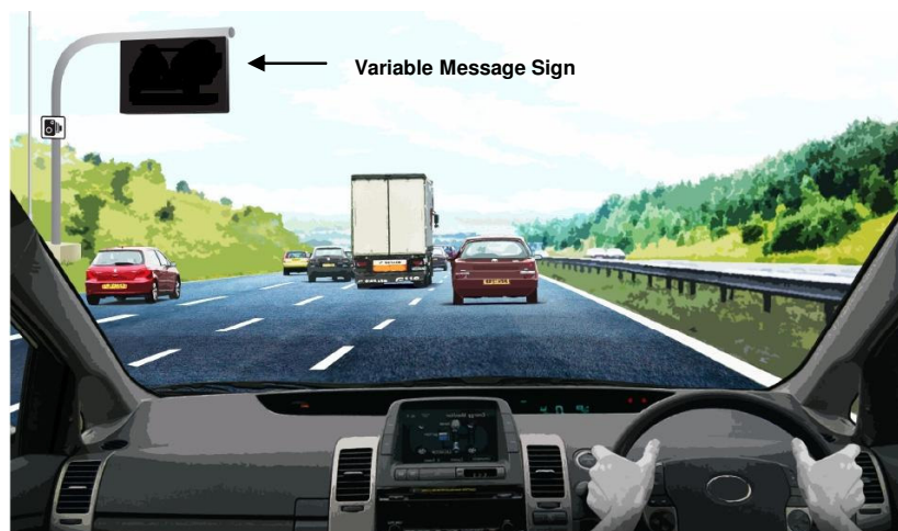
Figure 4B: Illustrative M25MM section operating in normal motorway conditions with a blank verge mounted Variable Message Sign
