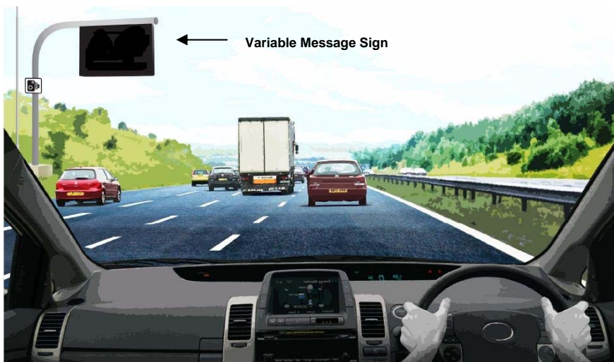
Figure 4.2D: Illustrative M62 J18 to J20 of the smart motorway all lane running section of the smart motorway scheme operating in normal motorway conditions with a blank verge mounted variable message sign
