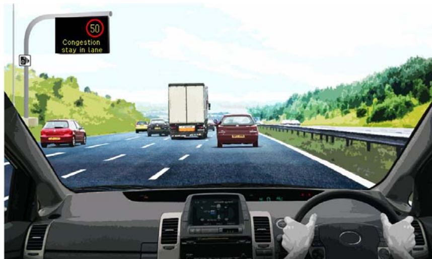
Figure 4.3D: Illustrative M62 J18 to J20 smart motorway scheme section operating with variable mandatory speed limits and information for road users.
