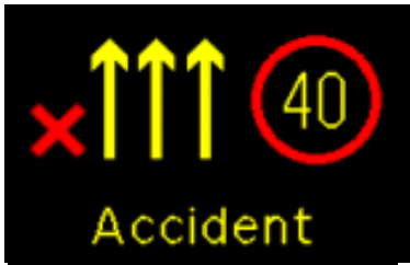
Figure 4.4C: Variable message sign warning of a closed lane ahead due to an accident
