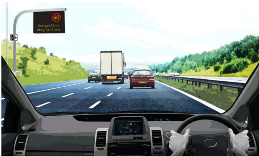
Figure 4.3B Illustrative M60 J8 to 18 controlled motorway section of the smart motorway scheme operating with variable mandatory speed limits and information for road users
