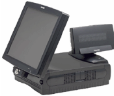
Figure 36 Toshiba ST-71 with integrated customer display unit
