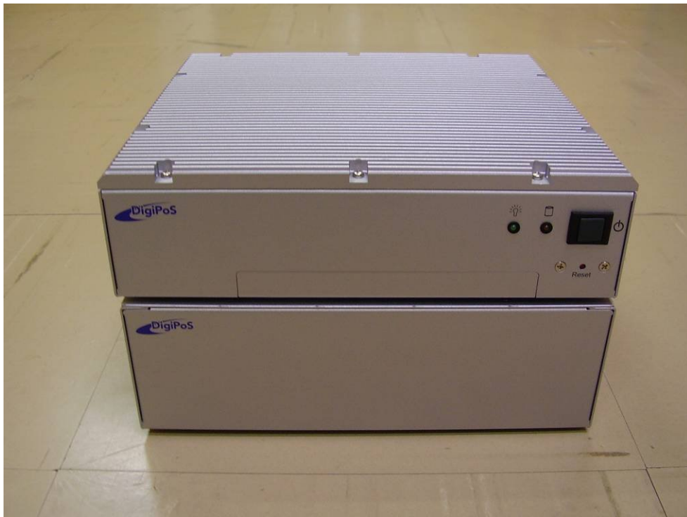
Figure 41 Front view of PH6000T System Unit showing Main system unit (top) and IO Expansion Hub (bottom)
