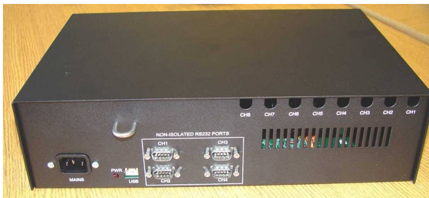
Figure 15 HTEC pump interface 950-00210-100: rear view showing connections
