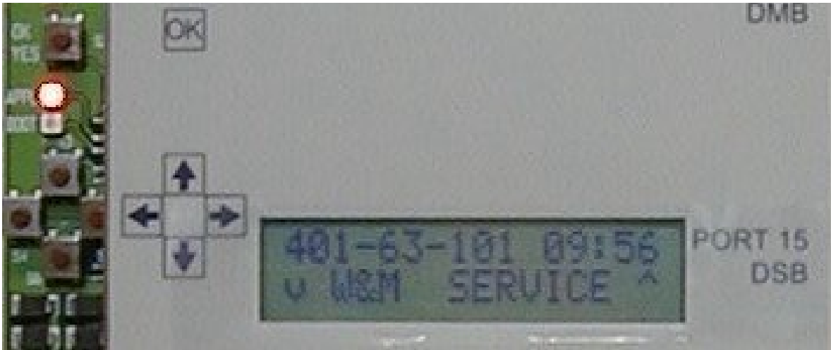
Figure 44 Central Processing Board (CPB508) display and menu navigation keys
