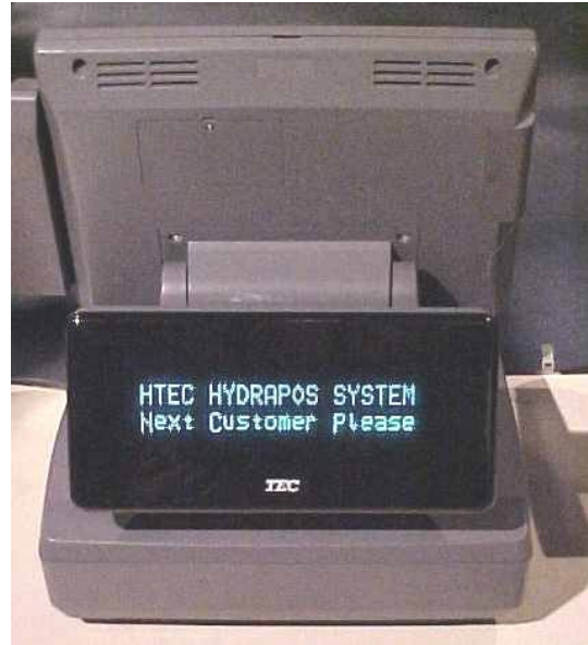
Figure 29 Toshiba TEC ST-70 POS unit showing kiosk display and customer display
