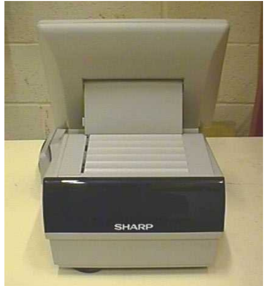
Figure 25 Sharp UP5900 – rear view showing integrated CDU
