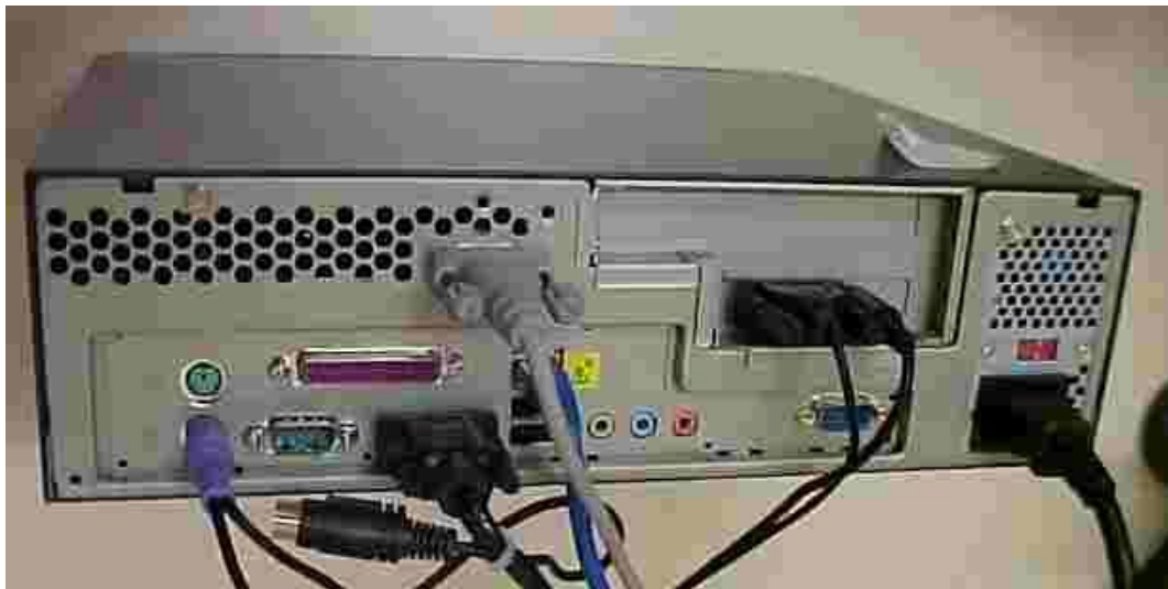
Figure 28 Epson MR800 POS unit – rear panel – cover removed note: pump control connection (not shown) goes to USB port
