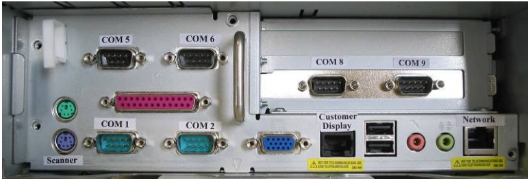
Figure 34 Epson IR 700 – showing rear connections with protective cover removed
