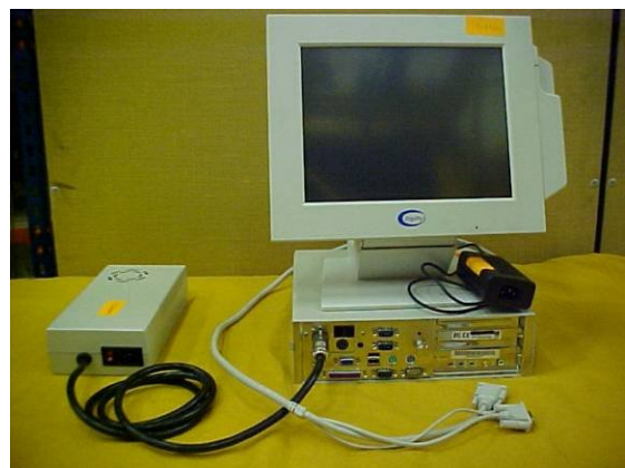
Figure 23 Front and rear views of Digipos 'Millennium' showing external power supply and rear connections
