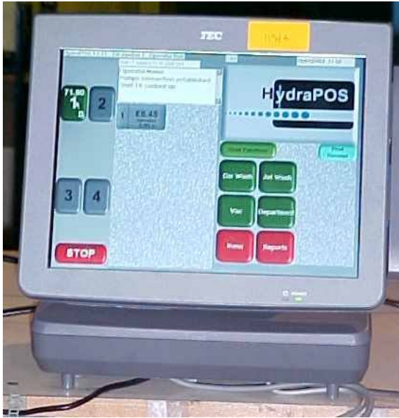
Figure 29 Toshiba TEC ST-70 POS unit showing kiosk display and customer display
