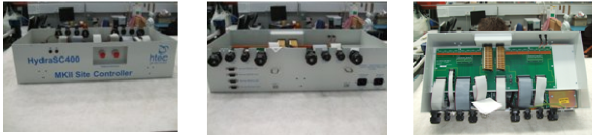
Figure 52 HTEC Hydra SC400 MkII site controller, part number 950-00251-100 (Resilient) also termed EC resilient site controller
