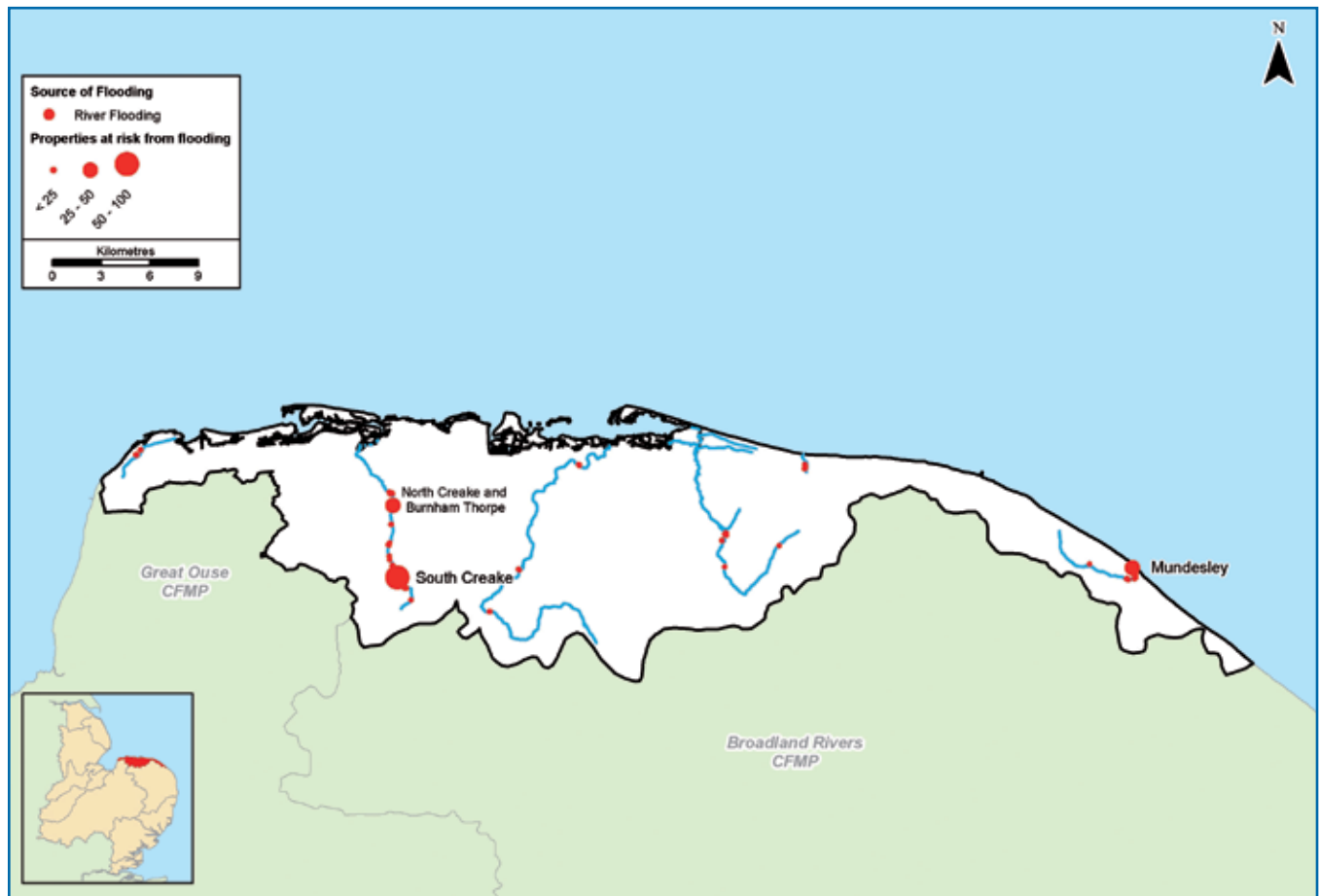
Map 2 Flood risks to property in a 1% annual probability river flood, taking into account current flood defences
