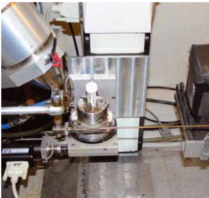
The new microscope in action: the X-ray generator is on the left, the specimen for examination is in the middle and the lead-lined camera is on the right.
