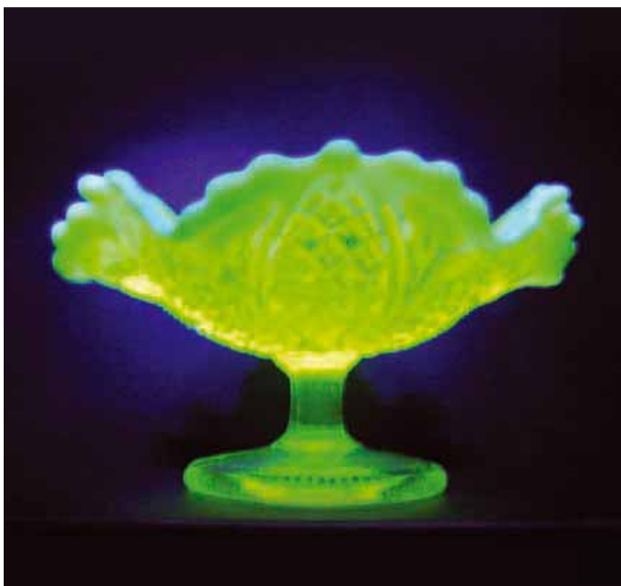
A uranium glass fruit bowl with the properties of fluorescence and radioactivity.
