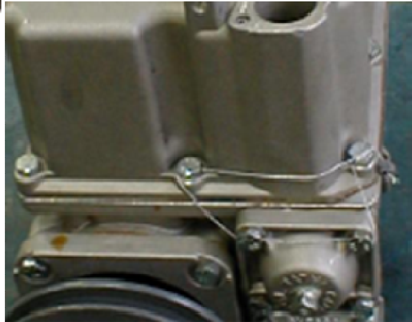
Figure 5b GPU-90 Pumping Unit Sealing
