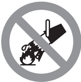
Do not extinguish with water
