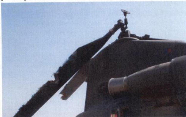
Fig 1-13 Aft 'Green' Lag Damper Failure
