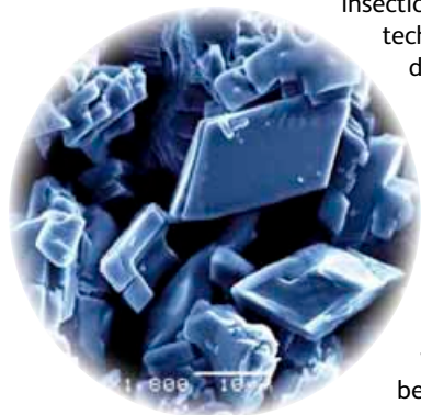
A magnified image showing the micro-encapsulation formulation of insecticide and synergist into a crystalline structure
