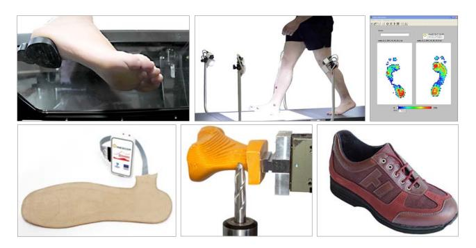
The scanner, gait analysis system, sensor system, machining process and finished bespoke Sshoe.
