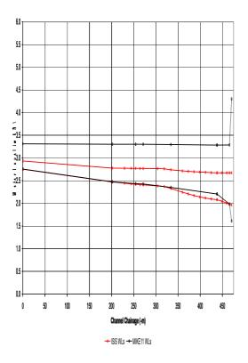
Graph 9 - Testi H: Comparison of Calculated Discharge Profiles at 20hrs
