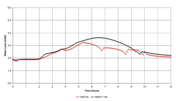
Graph 16 - Test H: Comparison of Water Levels at Control Point for Pumps
