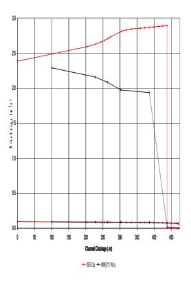
Graph 80-Test H: Comparison of Calculated Discharge Profiles at 0.0hrs
