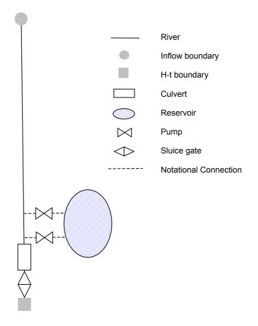
The model comprises cross-sections and interpolated sections along with a culvert, reservoir and a downstream tidal exclusion structure. Additional interpolated sections have been used as specified below for each software package.
