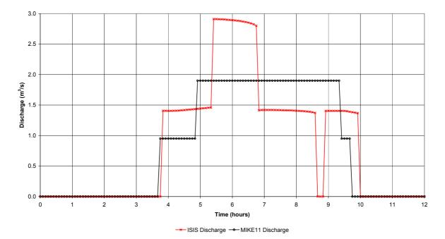
Graph 15 - Test H: Comparison of Calculated Discharge into the Reservoir
