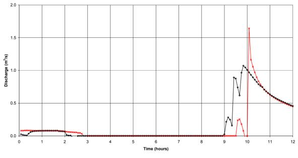
Graph 17 - Test H: Comparison of Calculated Discharge at the Downstream Structure
