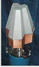
germanium crystals, each about the size of a baked-bean can. However, AGATA differs in that the germanium detectors fill up the entire sphere, which dramatically improves the detector's sensitivity. The paths of the gamma rays, as they bounce around inside the detector, can be reconstructed using state-of-the-art computer methods. This enables the researchers to record both the position and energies of all the gamma rays reaching the detector.
