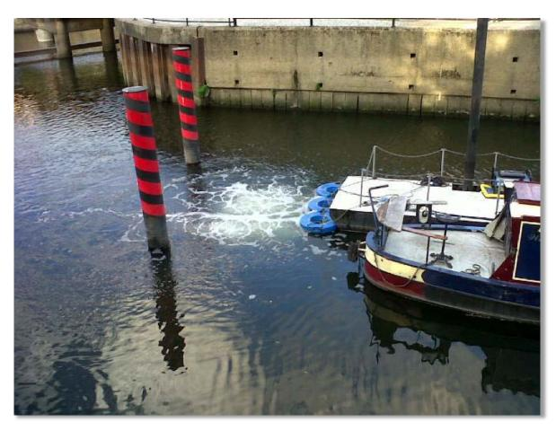
Aeration equipment was used to boost oxygen levels on the River Lee
