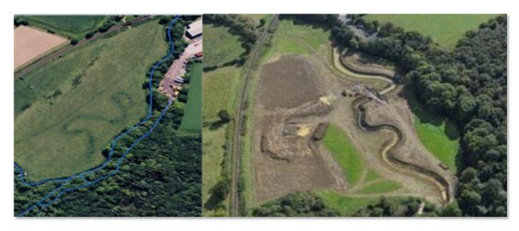
LEFT: Before MORPH - the river (blue lines) had been straightened, widened and given steep banks for navigation in the past. The old meander (wiggle) in the river is visible in the field. RIGHT: Photo taken during the works. The river has been re-meandered and brought back through the field. This creates different flows and habitats which will bring more wildlife to the river and slow the movement of water through the river.
