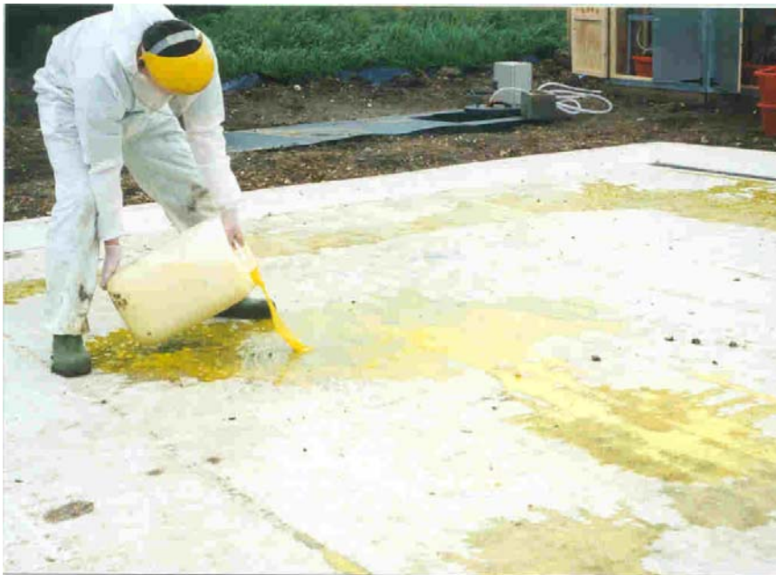
Figure 4.7: Application of sump rinsate mixture to concrete intercept
