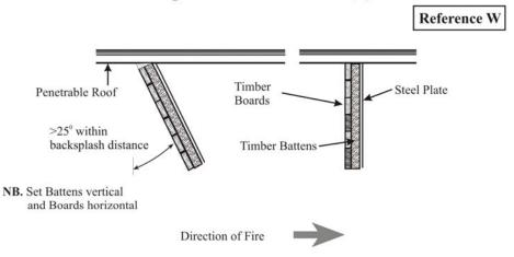
Figure 3-4. Baffle Construction
